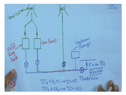
And when exactly this TiCl4 and H2, CH4, those are starts participating, in that case what we have, we have actually then TiCl4 plus H2 at the very beginning plus carbon from the substrate, we get TiC plus HCL. That is the first stage of this deposition. And it will follow this stage, TiCl4 plus CH4 and some hydrogen, so it will give us TiC plus HCL. Of course, we have to balance this thing. So this will be the reaction.
