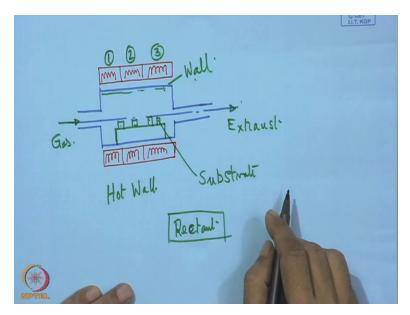
So what we can see here, hot wall reactor. So we can have just a very simple diagram to show this. Say this is one horizontal tube like thing and this can be either hot wall or cold wall reactor. Now since it is hot wall reactor, we must have the heating elements here. These are the heating elements. And we can have segmentation, that means this is one heating coil, this one too. So this is just one annular thing, so this is also continuation of that coil.
