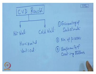
So deposition module is actually the reactor, CVD reactor now CVD reactor, we can have CVD reactor. One thing we can have say hot wall reactor, hot wall and then we have also cold wall. It can be horizontal, it can be also vertical. Now the question is, which one is the best? Now to address this question, what we have to tell here that the geometry of the substrate, it is actually geometry of substrate, number one.
