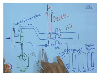
And now here what we have to connect, this can be, say in this case we can put one evaporator and this is just like a bottle. This is just like a bottle, so here it is blocked and what we have, we can have a supply of this liquid from this line. So this will be the supply line and this is actually the liquid and whose temperature is controlled by this heater.
