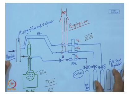
Plus this one what is the gas dispensing module, taken together that makes a complete CVD system.
