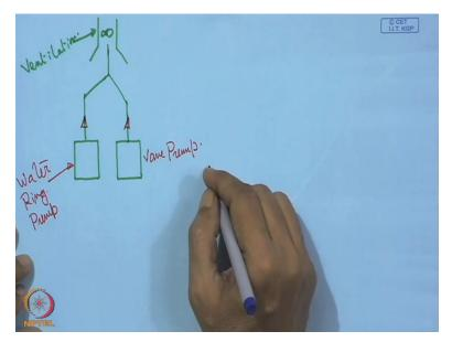
So from this point, what we have, here we have one, we can show symbolically two pumps operating in parallel, so they are connected. So this is actually ventilation. And one of this, that is called a mechanical vane pump, this is a vane pump. And this one is called water ring pump. This one is water ring pump and that is the vane pump. And that is the exhaust of this water ring pump and this is the vane pump. Now we have to have now the input.
