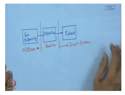
So here what we can see that we can have, say for example three modules are there. We can put this way. This is all gas dispensing, either gas or vapor, gas dispensing. So in simple language, it is gas supply. And then the whole thing goes here, what we call that deposition module, so this is actually deposition module. And then the last one, that is actually the exhaust. So we have all together these three modules: gas dispensing, deposition and exhaust.
