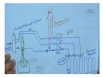
That means this, if we refer to that diagram, this entry point that will be very important where we are going to connect this line. So that is going to reactor, so how we are going to connect, whether it will be from the bottom and the gas will move up or whether it will be from the top to bottom, it will move vertically downward so all these things are to be considered while addressing this particular issue.
