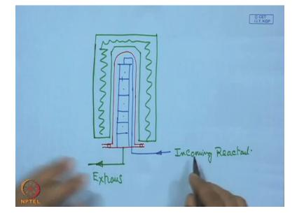
So for normal CVD what is done, it is mostly a vertical reactor. What we have seen normally, it is a flux and here what we have, this is the gasket and here we have a tower. So that means this is the tower. So this tower has various stages with perforations. So we have 1, 2, 3, 4, 5 stages and through that we have perforation. So here will be incoming reactant gas and which will be, which has an outlet and that will be connected on this side.
