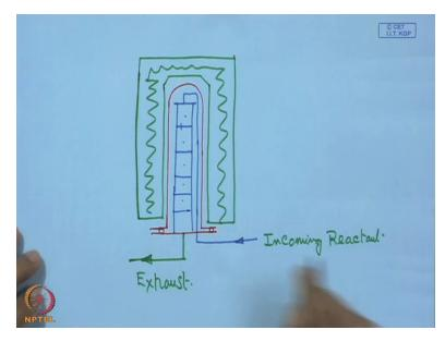
That means this is actually the coating deposition module which consists of the flux, the vessel, the CVD chamber along with a source of heat. It can be hot wall or it can be even radiant, in that case it can be a quartz tube and we can have some tungsten filament lamp for even heating that one. Now we go to this exhaust. Now what we have in this exhaust, we have to see that.
