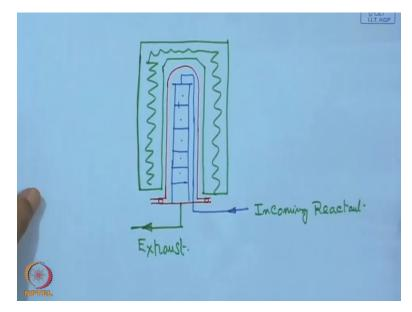
So this downstream module plus the module, this is the reaction module or the CVD reactor.
