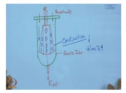
Say for example, we have a reactor of this fashion and here it is almost like a bell jar. So what we can do? We have a barrel, the barrel is placed like this. So this is the axis of the barrel. So this is actually a quartz tube. And here we have incoming reactants and that is the exit. So the barrel is something like this. So it will be, it has a shaft which is extended outside. So this will have a rotary motion. And here we can put the substrates.
