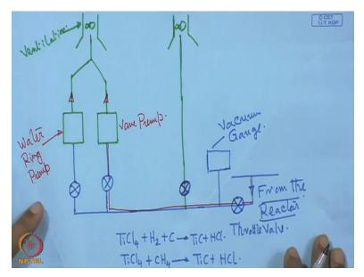
So when we have HCL, that means if we allow this HCL to pass through this vane pump, then this pump will be corroded and it will be damaged.
