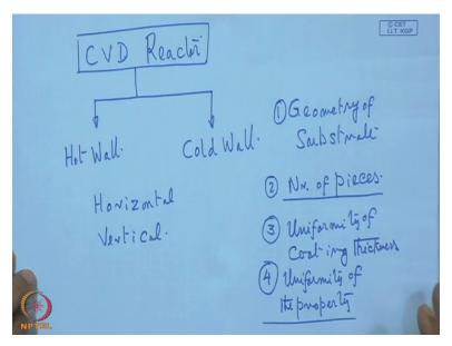
And fourth one, obviously uniformity of the property uniformity of the property, coating property, coating quality, uniformity of the property, these are at least one has to look. Geometry of the substrate, whether it is simple or complicated? Number of pieces means mass production or small batch production uniformity of the thickness and uniformity of the property. Now in this respect, we can also say horizontal, vertical, hot wall and cold wall.
