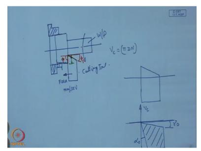
Now if this picture, if we redraw it here little in a bigger scale, we can see that this is actually the section if we take this section here we can find that, so this is actually the direction of velocity and this is a line perpendicular to that velocity, so this we call orthogonal rake and orthogonal clearance. So these are the basic thing for any cutting tool to understand the role of this coating. Now this particular tool is actually removing the material as it moves.
