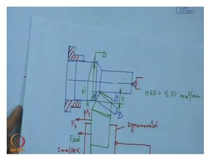
This face, this figure, here the chip will flow in this direction and as a result of this we can expect this tool, here this is the angle, this is called the principle cutting edge angle we have already described, this is the auxiliary cutting edge angle.
