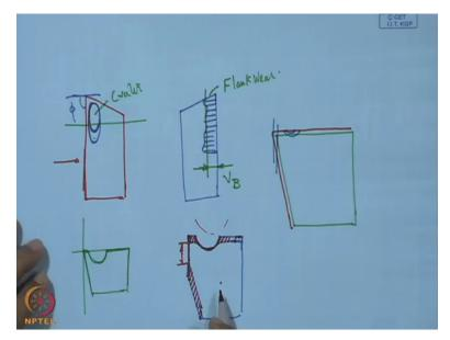
So here the principle cutting edge angle we have considered as 90 degree, whatever may be the case, now as the chip is moving, we can also have a crater like thing over this surface, now with this cratering cavity formation and this wear (())(51:23) formation on the flank, the tool will lose its cutting capability so this width will be actually equal to the width almost coming very close to that because the contact zone is equal to the width of the chip.
