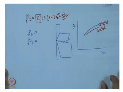
And then by this mathematical relationship it is also possible to find out what is the actual force which is prevailing here and which will be a function of this PX and PZ and since PZ and PX can be brought down by this mu, so naturally that friction force can be also reduced. So this way we understand that the cutting force is an indicator of good machining or poor machining.
