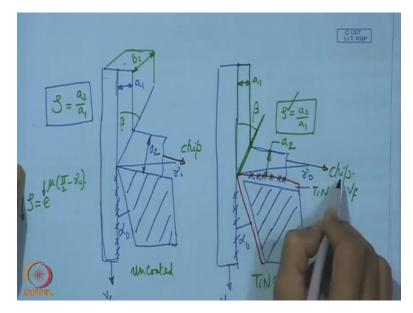
Here looking at this diagram in this here, what we have shown just now that here in this zone if we lower the friction then the friction force that means the drag force necessary for moving the chip in this direction that will be also reduced in comparison to what we expect here, it is because of the coating.
