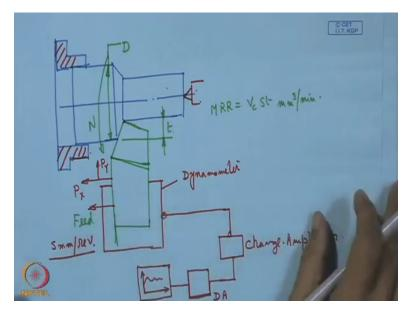
And also from this measurement PZ, PX, PY, which can be directly measured from this dynamometer because this dynamometer has three crystals so they can record directly PX, PY and PZ.
