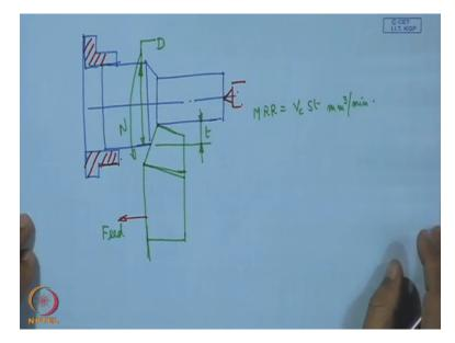
Now comes the cutting force, now cutting force means when we are using this tool, say a tool is being used like this, this a turning tool, and here we have the job like this, this is the work piece and here, so this the job holding device. So this is the cutting tool, now this cutting tool can be engaged for measurement of the force, so this can be used for collecting the chip and measuring the value of chip thickness and at the same time it can be also used for measurement of the force.
