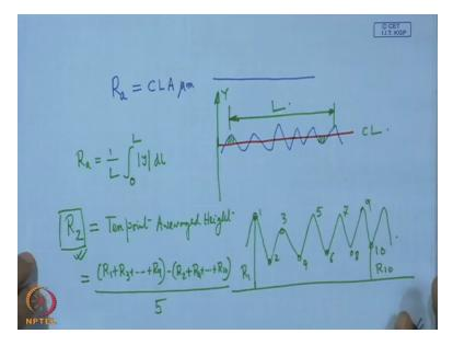
We have actually three parameters that has to be specified. Number one, what we call and it is the RA that is the symbol that is called center line average, center line average and which is expressed in micron, micrometer and this we can explain actually surface is not just like an optically flat planer surface.
