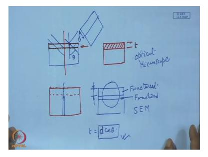
Micrography means in this case what we can show, this is just on the top we have the coating, so this was the substrate, original substrate and on that a coating is deposited. Now this coating can be visualized by microscopic examination, so one has to take a section of this one and then looking from this side, that means this is the cross-section which appear to be like this and this can be well measured under a microscope this thickness and here it is actually a metallograph.
