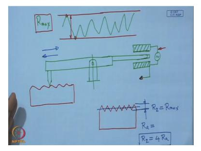
Now one such instrument, the basic principle we can show like this, this is basically one horizontal arm of that instrument, and this arm it is actually pivoted at this point, this is the pivot and here we have the stylus and this is mostly a diamond stylus and on this side what we see here it is actually one capacitance it is a capacity transducer.
