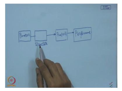
It is process then structure that gives the property and finally the performance. So what is important here to know what I exactly what I mean by the structure of the coating, architecture of the coating and there are various issues we have to look and properly address if those conditions and qualities are not properly made or satisfied so that is why this physical characterisation of the coating that is so important before we go to the next step. (Refer Slide Time: 2:22)
