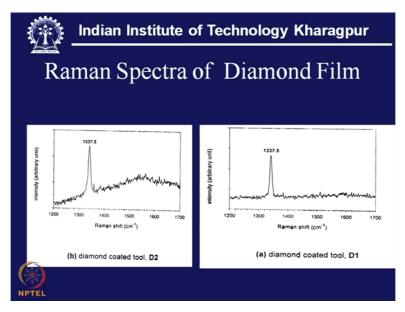
Now come very important tool and it is actually this Raman spectra. Now here this is very very useful if one is engaged in deposition of diamond coating, there are numerous use and application of this Raman spectroscopy but when it is a hard coating or super hard coating one can just go for use of this Raman spectroscopy with a very clear objective.
