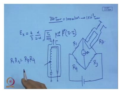
And so there is one equation and what can be written as E k that means the heat loss due to this conductivity it is given by alpha by 2 - alpha root over T 0 by 273 into so here we find that this is called accommodation coefficient, this is the molecular thermal conductivity,
