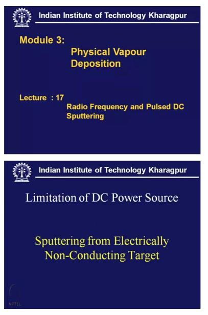
Radio frequency and pulsed DC sputtering, this topic we are going to discuss today. Now why do we need this radio-frequency sputtering or pulsed DC that means in this case the power supply will be available at a sinusoidal form that means this voltage which will be supplied to the electron that will keep on changing with the time and this frequency will be very high order and why do we need it? Normally DC sputtering is well-known for well-
