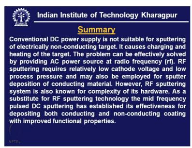
So with that we come to the summary which can state and be stated as conventional DC power supply is not suitable for sputtering of electrically non-conducting target. It causes charging and heating of the target and finally lead to arc discharge stopped this problem can be effectively solved by providing easy powers so is at radio-frequency which is in the order of 13.56 megahertz. RF sputtering requires relatively low cathode voltage and low process
