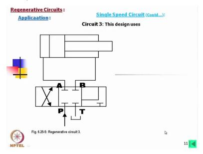
Now circuit 3; in this case before writing this what is this valve? 4 by 3 valve, this is 4 by 3 DC valve okay. Now when the spool is in neutral condition, all the ports are blocked so there is no motion. During the right solenoid operation, regeneration takes place that means here the in the valve itself the regenerative circuit is made, it allows the mix this oil with this one, but when it is sorry this in the other position which I have not shown that is that will give the normal return okay.
