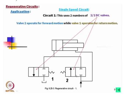
Now this circuit, we will discuss few circuits, in this circuit we have used this we have used 2 DC valves 2 by 2 DC valves, definitely you understand as you know the symbols that 2 by 2 DC valve. Then how it operates, valve 2 operates for forward motion that means and valve 1 operates for return motion, let us say valve 2 is engaged that means the flow is going like this okay, this is
