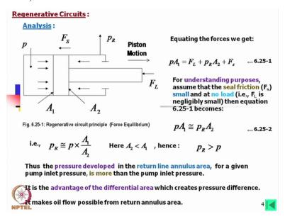
Now we can use this force, P into A 1 that is full area must be equal to FL = PR into a 2, whatever may be this pressure = F s the friction force okay. For understanding the purposes of the regenerative circuits circuit how it works, let us assume that friction force is negligibly small and we shall also equate this at no load, then equation 625-1 becomes P A is equal to P R into A
