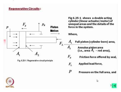
Now in this figure we find a double acting cylinder linear actuator motor we can say linear actuator motor of unequal area and the details of the force in the system. Now I would say that if you remember this term double acting, double acting means its acting in both way, it can do work while it is moving in former direction, also it can do work while it is in the written motion. However, in most of the cases you will find the return load is usually less it is mostly less.
