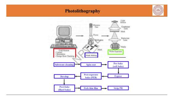
So, the light falls onto the mask and passes through the mask and thereby whatever features on this mask are made for blocking the light would block those portions of the light and whatever features are open are open and light passes through them and falls onto the wafer which is actually coated with the resist.
