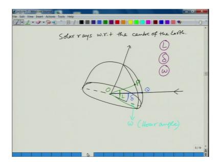
And then another set that we have learnt is the solar rays with respect to the centre of the earth ok. So, we have seen that the earth rotation axis is at certain angle with the orbital plane.
