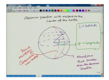
So, what else have we seen is the observer position with respect to the centre of the earth ok. This we have already seen that if this is earth ok and if we have this is the centre and we have this equatorial plane. So, if observer is here ok on this particular position, let us say this is P, so the angle this particular line makes with the equatorial plane that is our latitude. So, L is the latitude.
