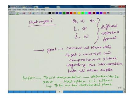
So, what angles we have seen so far? Theta z, alpha, A z. And from the next figure, what we got the latitude and phi or the latitude and longitude ok. And then from the other figure we have seen another two angles; one is declination angle and hour angle. So, one is declination angle and hour angle ok.
