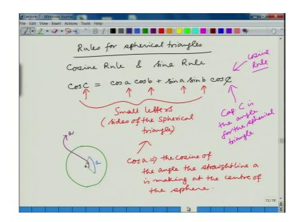
So, rules for spherical triangles. So, rules for spherical triangle is one is called cosine rule and the other one is sine rule. What is the cosine rule is this one cos c ok, we will talk about it in a while cos c equal to cos a cos b plus sin a sin b and cos capital C ok. So, what is happening here, what is going on? These are all small. So, let me say this, this, this, this and that are all small, small letters ok.
