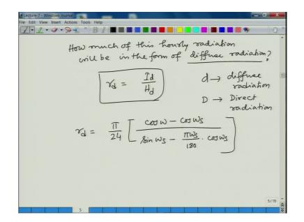
Now, one small piece of information is still left which is how much of this; how much of this hourly radiation will be in the form of diffuse radiation right that is a legitimate question to ask. And the complementary part will be given or complementary part will be the direct radiation right.
