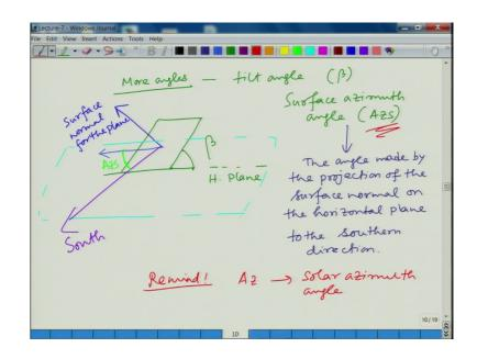
So, more angles that we need that are needed is the tilt angle right which we call beta. So, what is that if you have a planar like collector, what angle does it make with the horizontal? If this is the horizontal plane ok, the angle it makes is called the tilt angle. So, that is one important angle we need to consider. And also whenever you have a plane, then you can draw a surface normal for that plane right. So, this is surface normal for the plane.
