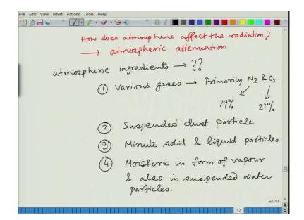
Now, how does atmosphere affect the radiation? That is the question we are going to look at now. And it is often called atmospheric attenuation; because, it will actually attenuate or reduce the intensity of the solar radiation that is why it is called atmospheric attenuation ok.
