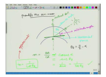
So, quantify the air mass ok. So, now, let me draw that figure again or maybe just the atmospheric part. So, here we have CB and A ok. And this is what can you tell me? This particular plane this is the horizontal plane right, because this is the center of the earth ok. If you connect that to the observer location and extend that this is the vertical direction.
