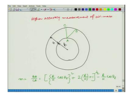
So, if you want higher accuracy so higher accuracy measurement of air mass that would require the curvilinear path between B and A ok. So, in that case what we can. So, let me draw it first because the curvature we need to consider, we need to take what are the values of if this is the radius of the earth, and if this is the height of the atmosphere H and R, then you can get then other things stay the same this is BC and A.
