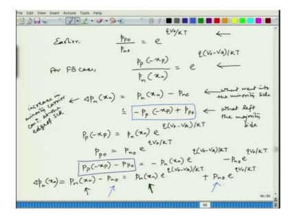
So, earlier what we have seen is this under equilibrium what are the ratio of carrier concentration across the space charge region, ok. So, hole concentration ratio between P side and N side is,
