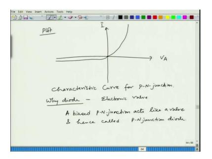
So, now, if we plot this common function, how will it look? In this direction we have I and in this direction, we have  $V_A$  (applied voltage). So, you have seen the forward bias part will be like this right and the reverse bias part will continue and we will have a constant reverse saturation current  $I_0$ , ok.
