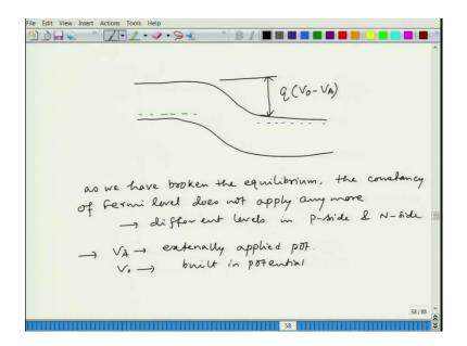
So, you have this thing. Now, you have reduced it to a lower value. So, basically this is the potential barrier or equilibrium, we call it built in potential. Now, we have this energy barrier, which is less than the built in potential, because we have applied the potential in such a direction that the effective potential gets reduced and that is called forward bias. And now, as we have broken the equilibrium, we are no longer under the restriction of constancy of fermi level, ok.
