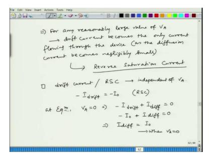
So, for any reasonably large value of applied voltage, the drift current becomes the only current flowing through the device as the diffusion current becomes negligibly small, ok. Now, this value of drift current that is independent of the bias we call it reverse saturation current, ok.
