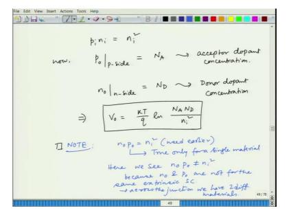
And this  $p_i n_i$ ; we have seen earlier that it is  $n_i^2$ Because  $p_i$  is equal to  $n_i$  for intrinsic semiconductor ok, now, if we look closely at the extrinsic value, the  $p_o$  in the p-side that is what depends on the concentration or that is equal to the concentration of ionized acceptor donor.
