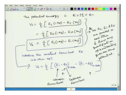
And we have also quantified that quantity which is the built-in potential, and that depends on the distance between the intrinsic and extrinsic Fermi level in the P-type and the same for the N-type ok. So, here this  $E_i$  stands for the intrinsic level or intrinsic Fermi level, and this  $E_F$  stands for the extrinsic Fermi level. So, we quantified it in terms of for the; the first term here is for the P-side and the second term here is for the N-side ok.
