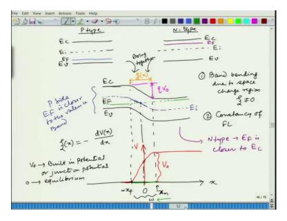
So, this was the picture we have seen in the last class, right, and this built-in potential  $V_0$  in the equilibrium potential, which is just obtained because of this close contact of two types of semiconductors ok.
