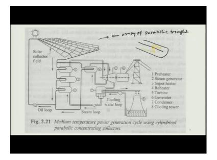
So, here you can see this is an array of parabolic troughs. So, how do they look? You have the parabolic surface, which is long, and at the focal point, you have the tube which carries the fluid and gets heated by the collector ok. So, what is happening here? You have these solar rays are falling on this and then getting reflected onto this focal plane, where the pipe is running; that is how the parabolic trough collector works.
