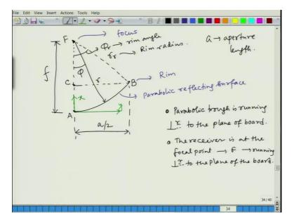
Now, if we do the optical analysis of that first thing, we can draw that let us see that this is the parabolic surface, and this is the point of focus. So, let us say this point to be F and the midpoint of that surface, I am just drawing half of it, and the other half will be symmetric so, if this is the parabolic surface, parabolic reflecting surface. And, this is the focus of the parabola. Now, let us say that B is the endpoint of it so, this point B is called the rim.
