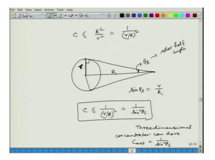
So, in the last class what we have seen? The three-dimensional concentrator can have  $C_{max} = \frac{1}{sin^2(\theta_s)}$ . That means that is the  $\theta_s$  is the half-angle that the solar disk makes on the surface of the earth. So, these  $\theta_s$  let me just repeat that it is the half-angle the solar disk makes on the surface of the earth. And for 3d concentrator, we have  $C_{max} = \frac{1}{sin^2(\theta_s)}$ .
