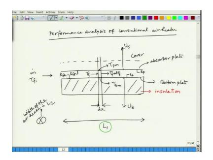
So, this is the figure we drew in the last class where we have seen that we have a cover and then we have the absorber plate and then we have the bottom plate here, ok. And the lower portion is insulated and we have seen that the resistance circuit, the thermal resistance circuit is little bit different in this case.
