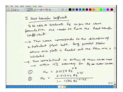
So, a note on the heat transfer coefficients, ok. So, to be able to evaluate  $F_R$  as per the above formulation, one needs to have the heat transfer coefficients right and this case actually corresponds to a known case from the convective heat transfer coefficient or convective heat transfer theory. This case corresponds to the situation of a turbulent flow between long parallel plates where one plate is heated and the other one is insulated, right.
