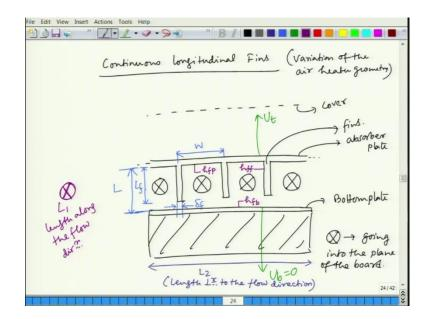
Now, we are going to look at one other very common variation of this air heater where to increase the heat transfer area what we do? We use fins to increase the area and those are continuous longitudinal fins, ok. So, this is kind of a variation, but very common variation of the air heater geometry, ok. So, what do we mean by these continuous longitudinal fins?
