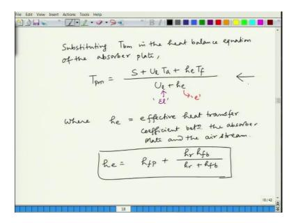
So, if we do that by substituting  $T_{bm}$  in the heat balance equation of the absorber plate, what we can write? We can now have a much simpler expression for the mean absorber plate temperature, ok. What is that? It is
