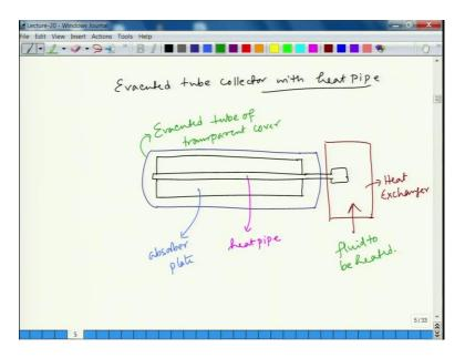
So, evacuated tube collector with heat pipe, I assume that heat pipe how it works you are familiar with the concept. The heat pipe is nothing but a pipe where natural convection is used, and the phase transition is also accomplished.
