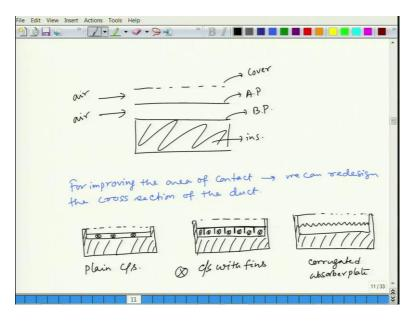
So, that is one variation you can have, and you can also have the cover. Now, you have the plate, bottom plate, and cover everything you have. This is insulation, this is the bottom plate, this is absorber plate, and this is cover, and you can also have the airflow through both these portions.
