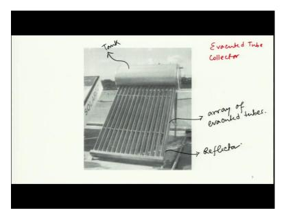
So, here we see an evacuated tube collector, so, this is an evacuated tube collector, which is more often than not, you will see these kinds of configuration in the rooftop solar heaters. So, here what is the different portions? So, you can see this is the tank, and this is the array of evacuated tubes. So, each tube will look like the one that I just showed, and at the back, you have some reflector. So, this is a typical evacuated tube collector.
