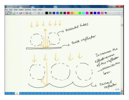
Coming back to the reflector, if we look at it a little more closely, what we can have like you can have one configuration where you have this reflector at the back, and you have these different tubes. So, these are evacuated tubes, and this is the back reflector.
