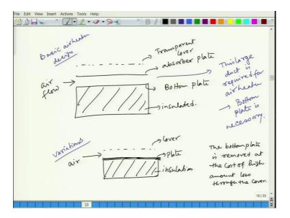
So, typically what we do have, we use two plates: one is the absorber plate, and another is the bottom plate. So, suppose we have this is the absorber plate and typically what we have? The cover, transparent cover here. Now, as the volume flow rate is high, we need a bigger channel or bigger duct through which the air is flowing.
