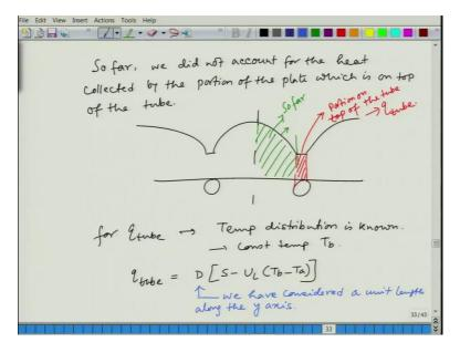
Now, so far, we did not account for the heat collected by the portion of the plate which is on top of the tube that is carrying the fluid. So, that means, what do I mean? We have this plate; we have these tubes; we have seen that the temperature profile will be somewhat like this and what we have accounted for is the heat collected by this portion. This we have accounted for.
