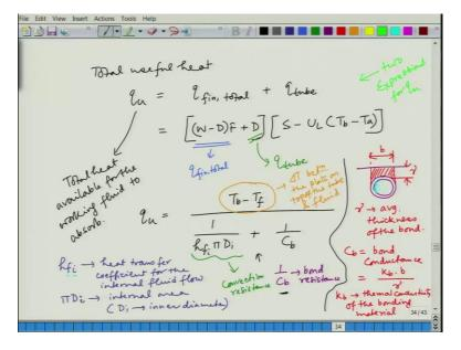
So, what can we write? Now, the total useful heat that is heating up the working fluid that is
