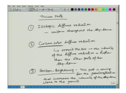
So, we divide it in three parts ok. 1st one is we call isotropic diffuse radiation what is isotropic? You mean isotropic means, it is same in all direction that is what the term isotropic mean. So, this is the part which we assume that uniform throughout the sky dome ok.
