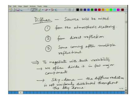
So, first let me talk about the diffuse radiation. So, for diffuse radiation, the source will be mixed, it would not be a single source ok. So, what would be the sources? 1; from the atmospheric scattering, then from direct reflection from some other body ok and some coming from or coming after multiple reflections.
