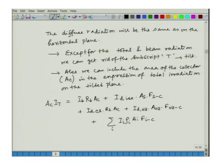
So, one thing we notice here the diffuse radiation will be the same as on the horizontal plane right. Because horizontal plane I mean the diffuse radiation does not have a definite direction right. So, that is why it does not depend on the angle of inclination or the tilt of the plane ok.
