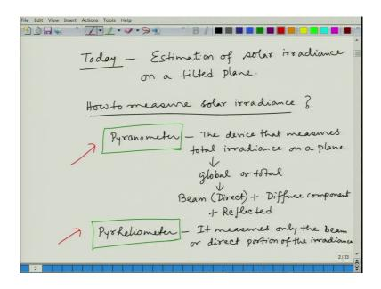
So, today what we are going to discuss is the estimation of solar irradiance on a tilted plane ok. So, this is a very vital topic which tells you how much solar energy will be available to your collector and often these solar collectors are placed in a tilted position, tilted to the horizontal plane ok.
