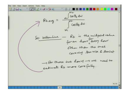
So, what we need to do then? We take an average value of R b corresponding to the whole period ok. So, we integrate the tilted plane incidence angle cosine of that throughout the available period of solar radiation and we do the same thing for the zenith angle and take the average, then it is not a single midpoint value, but it is the average of the whole illuminated hour that is how we do this ok.
