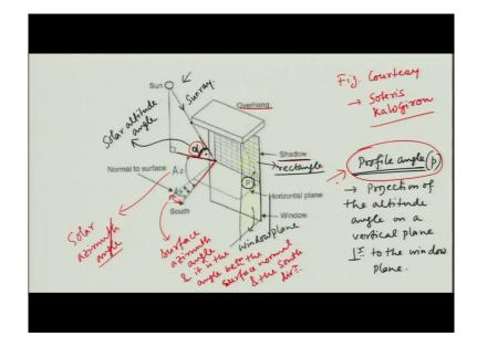
So, let us look at it ok. So, this is a much cleaner picture of a overhang on a window and it also tells you several of the important angles that we are looking at ok. So, this is our overhang and this is the shaded portion that you see that is the shadow it makes on the window or the wall ok.
