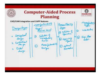
So, if you look at it, so we have a design layer, we will have a manufacturing layer, then we have a process plan, process planning layer, and then we will have again a manufacturing layer. So, this one is manufacturability layer and which is nothing but a macro layer, at a macro level. So, here you will have conceptual design, a, you will have embodiment layer or design, b, c, you will have detailed design, these are all the design layer.
