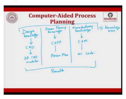
So, if you want to put the Computer Aided Process Plan in a schematic diagram, we have design knowledge, this leads to CAD system and this goes to 3D CAD modeler. So, this is one vertical, next is process planning knowledge, this will lead to CAPP Computer Aided Process Plan and this gives you a process plan. The other one is manufacturing knowledge, this goes to CAM, and this goes to NC code.
