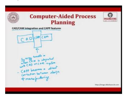
So, here let us just see CAD here, this is CAD, where we have studied all the graphical thing, then we have a CAPP here, then we have a CAM here. So, the function of a CAPP is going to be it gives you a synergy results in when CAM is integrated with CAD or CAM system. So, CAPP becomes a direct connection between design and manufacturing. So, this is the way CAPP features in between CAD and CAM, this is very important.
