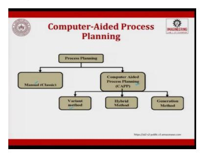
So, whatever we have studied till now, if you want to put it in a block diagram, we have a process Plan, which is manual process plan, and when the Computer Aided Process Planning, the Computer Aided Process Plan. Now, is classified into variant, hybrid, and generative.
