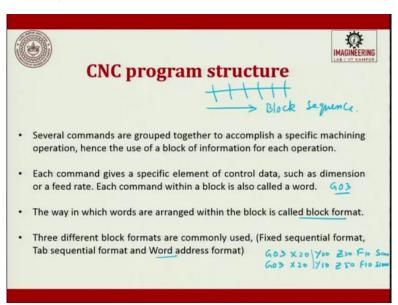
Several commands are grouped together to accomplish a specific machining operation, hence the use of a block. As I said, a line of information for each operation. Each command gives a specific element of control data, such as dimension or feed rate. Each command within your block is called a word. So now, G03 is a word. The way in which words are arranged within the block is called as a, block format. So, I said, a line. So, what has to start and how it has to end.
