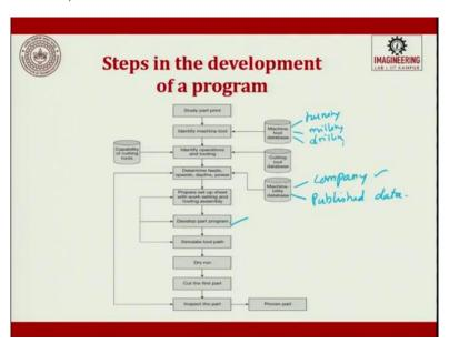
So, the steps involved in developing a program. First, study the part, identify the machine tool, so the machine tool database which is turning, milling whatever, drilling you will see that. So, machine tool identification. Then, identification of the operations and tools, so tools come from here, operations come from here. So, capability of cutting tool and cutting tool database comes from here. After this is done, then you try to look at the feed speed, the depth of cut power required.
