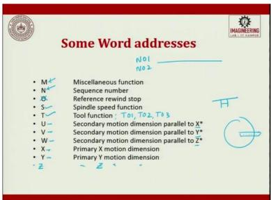
So, some of the words which are used A, so it is a rotation about X is A, B, C. Please understand the logic only here, and A, B, C can be changed from controller to controller. It can be alpha, beta, gamma, it can be u, v, w. So, look at the controller and then see what is it.
