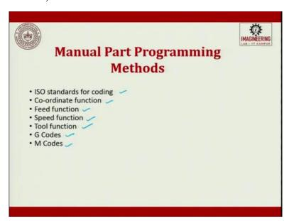
So, when we talk about manual part programming methods There is ISO standard codes available, the coordinate functions. Then you will have feed functions, speed function, tool
