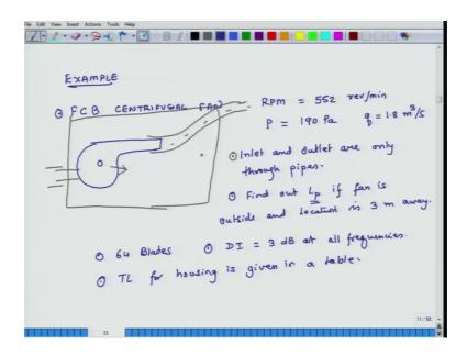
So, what does the what is the question that suppose, we have a forward curved blade type of centrifugal fan. So, we have this type of a fan. So, we know, what type of fan and it is rotating at it is r p m is 552 revolutions per second; it is revolutions per minute that is the
