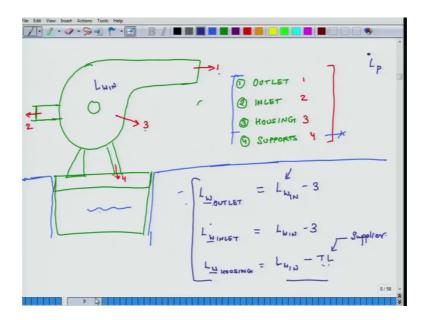
So, once again I will draw the picture of a fan or actually blower. So, that is it is sitting on a foundation. It also has an input inlet, this is the outlet. So, the four pathways we had discussed were outlet second is inlet, third is it can come out through housing. So, this is. So, this is 1, this is 2, one this is two path the third path is through the housing. So, that is
