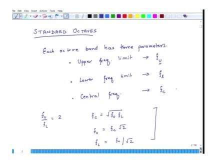
So, we will discuss standard octaves each octave band has 3 parameters the first parameter is upper frequency limit. So, this we designate as f subscript u and u is standing for upper frequency limit then it has a lower frequency limit and that is designated as f L and then it has a central frequency and there is a mathematical relation between all these 3 parameters. So, this central frequency is designated as f c.
