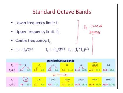
Where some of these bands are listed not all the bands are limited listed some of them. So, this is the central frequency for different octave bands. So, one octave band has a central frequency of 1, then the next band has a central frequency of 2, then 4, 8, 16, 31.5 and so on and so forth.
