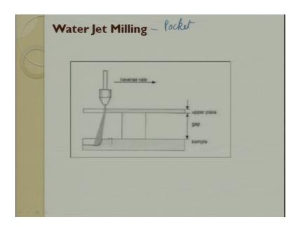
So, milling is basically what you are trying to talk about is to make pockets till now what we were seeing is only cutting. So, cutting means through to through cutting now what we are trying to talk about is how do you mill a surface to get the required output.
