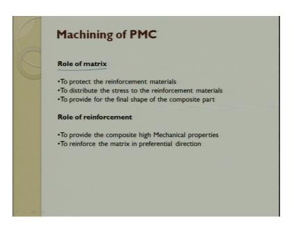
The role of the matrix which we have already seen so one is to reinforce the matrix material to distribute the load and to protect the reinforcement agent whatever it is to give a final shape, when you talk about reinforcement it tries to take the strength.
