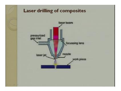
Going to non conventional the most popular one is glass fibre reinforce is laser drilling composite, in laser drilling composite laser beam photon lens, you reduce the diameter, there is a laser the laser jet comes and hits if you want you can also have a career media to gas to support and then try to make a jacket and then used for cutting.
