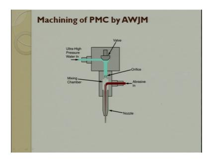
So, this is how it happens for a abrasive water jet machining. So, basically water comes in a very high pressure the there is a mixture mixing chamber. So, in this mixing chamber you can try to mix Abrasive water and then abrasive or you can try to have air and abrasive air and abrasive it is called as abrasive machining process water and air is called as water abrasive machining process. So, it comes out of the nozzle and then you tried to do a machining.
