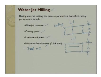
So, then it is more or less called as a abre or it is called as water jet milling. So, in water jet cutting the process parameter that affect the cutting performance are going to be pressure speed laminate thickness and nozzle diameter, when it goes to water jet milling the feed rate feed rate place a very important role and the feed rate is plays a very important role. So, you do not allow a through cut to happen and get the required output.
