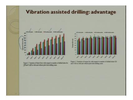
So, you can see the enhancement in performance of see the thrust force this is for vibratory assisted and the this is for non vibratory assisted. So, you can see the variation in the thrust force with respect to number of holes drill for CDUID these are a vibratory assisted drill and this is a conventional drill they have done and you see the response
