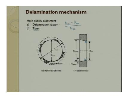
When you look at the damage which is created because of drilling so you can see that this is the diameter nominal I wanted and this is the diameter which the maximum damage diameter. So, this can be expressed in delamination factor which is nothing, but D max minus D nom by D nom. So, you will always have it in terms of ratio and this ratio we will try to maintain it as low as possible and if you see the delamination it need not be uniform all across it happens at several purchase.
