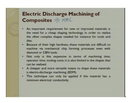
So, electric discharge machining of composites are possible wherever you want to do a metal matrix composite. So, there has to be a metal to finish the circuit.
