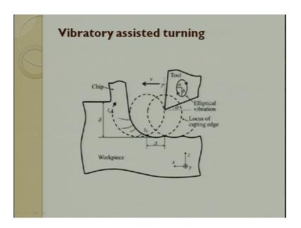
So, what people have done is people have thought of various ways. So, one way of doing it is in turning itself rather than having a continuous contact of tool and the workpiece what they said is why do not we try to have vibratory assisted turning. So, vibrate assisted turning vibratory assisted drilling is all used. So, what they do is they try to give a small vibration to the workpiece so the vibration can be along the z direction or can be along the xy plane.
