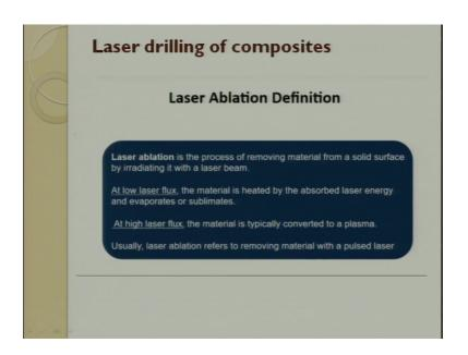
So, here in laser it is predominantly heat. So, it talks about the laser flux; laser flux is nothing, but joule per area. So, laser ablation is a process of removing material from a solid surface by irradiating with a laser beam, at low laser flux the material is heated by the absorb laser energy and evaporated or sublimated at higher laser flux the material is typically converted to a plasma, usually the laser ablation refers to removing of the
