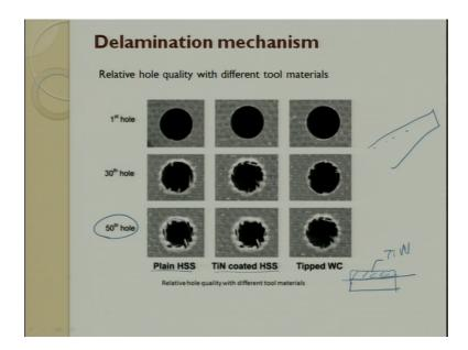
If you look at it the first hole thirtieth hole and 50th hole if you look at plain HSS because of the tool geometry getting distorted you see the fibre is not getting cut, but the fibre is pulled out of the matrix and it is left there. When you look at titanium coated; that means, to say I wanted to enhance the temperature wear resistance. So, I do a coating on top of this HSS tool and you see there is a slight enhancement, but it is not. So, in the first one it is second one.
