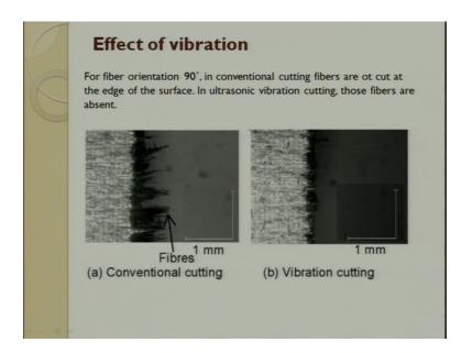
So, when you see that at 90 degrees you see there are lot of fibres which are getting pulled out and there is this fibre which is getting pulled out are not also cut properly, but whereas, when you see a vibratory assisted there is a proper cutting and the fibre pullout is not there see if there is a fibre pull out after doing an operation it is very difficult for you to trim the fibre and get the required output.
