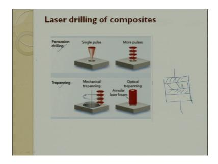
So, the laser drilling can be done like this you can do something called as a percussion drilling, you can also do a trepanning drilling trepanning drilling is you try to move around the around and generate a hole and then you do it step by step by step say for example, if you want to do a hole first you do up to here, then you do up to here, first this is the first layer, this is a second layer, this is a third layer, you can keep doing it and you move it in circles and get it done.
