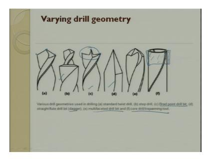
So, now you see here there are various drill geometry which have come into existence. So, these drill geometries make sure that the thrust force is reduced to a large extent, if you reduce the trust force the pushdown delamination can be reduced in a large way.
