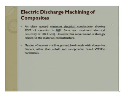
So, this is predominantly used for metal matrix composite and of course, if you can make a ceramic matrix composite conductive. So, then that is also used for machining. So, I have put down the properties which are there. So, minimum required electrical
