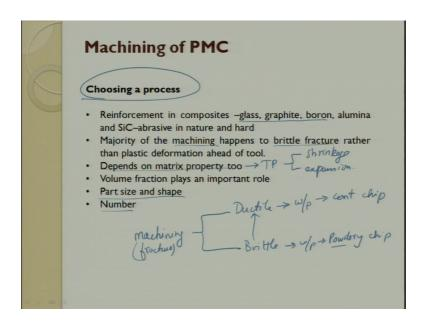
So, choosing a process the Reinforcement and composite can be glass, graphite, boron, alumina, and SLC. So, you have to look at the size shape of the reinforcement and decide your process. Majority of the machining happens by brittle fracture when you talk about machining there are 2 types of fractures machining fracture one is called as a Ductile fracture the other one is called as a Brittle fracture.
