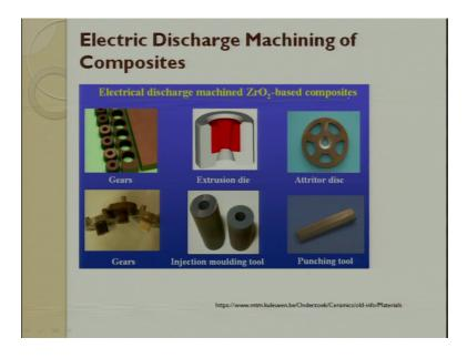
So, these are some of the electric discharge machine zirconium oxide based composites. So, these are some of the things which are made out of it and then people are using it.
