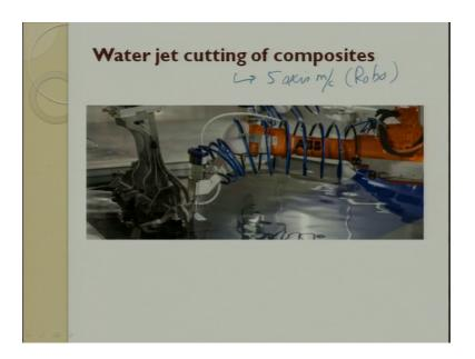
People have started using water jet and water jet also they have started using 5 axis, 5 axis machine and it is basically a Robo which is used in the hand of a Robo they have given a water jet, this water jet nozzle tries to move over a surface to make 2 D cuts.
