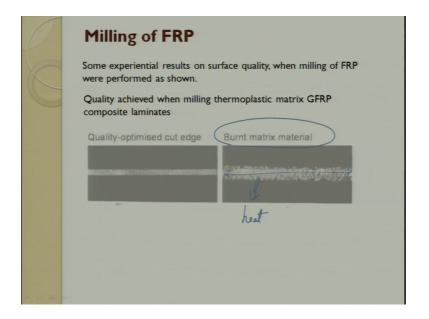
So, if you get a optimised cutting edge, if you want you can see this is the top view you can see a milling cutter is cut and then you can get a you can get a perfect channel made. If you try to use a burnt matrix material so what happens is there is a distortion which is happening along the running direction and the tool geometry is hit. So, some experiments results on surface quality when milling of FRP were performed as shown the quality
