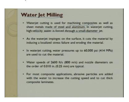
So, water jet milling. So, here the water jet cutting is used for machining of composite as well as sheet metals made out of steel and aluminium the water jet cutting has a high velocity water is forced through a small jet.
