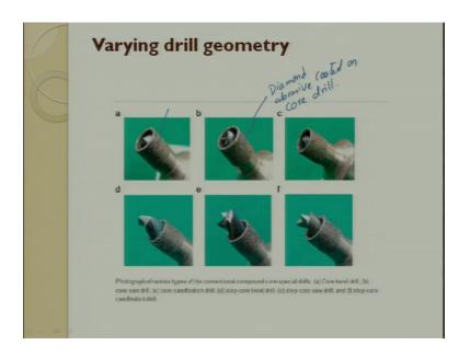
So, this is a figure whatever I was talking to you about. So, people have also tried to this is Diamond abrasives coated on on Core drill. So, you can on a core drill. So, core you can see a core twist drill you can see a core saw drill, these are core saw drill, then you can have a candle stick drill, then you can step cone drill. So, these are all different geometries today which people are using to reduce the delamination in a big way.
