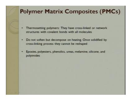
When you look into thermo set polymer they have cross linked or network structure with covalent bond with all molecules, they do not soften, but they directly decompose with heat, once solidified the cross link process they cannot be reshaped. So, the examples are polyester, epoxy, phenolic, furious and silicon are some of the examples of thermoset polymer, when we talk about the composite.
