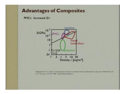
So, what are the advantage of polymer matrix composite? It has a very high e by r ratio. So, a r is the density or it can be considered as row, you can make it as row its row e by row is very important. So, you can see polymers fall in this region polymer matrix composites fall in this region ceramics much, ceramics much higher and metal alloys fall in this region. So, this makes polymer matrix composite more prominent for applications where weight is an important factor.
