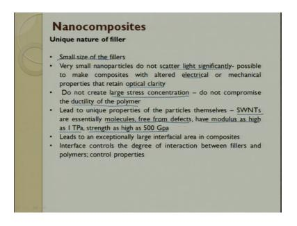
What is the unique nature of the filler which we use it is small in size very small nano particles do not scatter light significantly possibly to make the composite with an alt which alters electrical and mechanical properties that retains optical clarity. So, what we are trying to tell is we are trying to say electrical property and mechanical property can be can be changed by retaining the optical clarity; that means, to say you will have a
