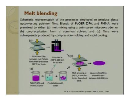
So, this is melts blending process schematic diagram. So, here you try to take the polymer and then what you do is you try to extrude it at 240 degree Celsius 100 r p m you try to do this and then you try to mix it up, you put it in a compression mould and
