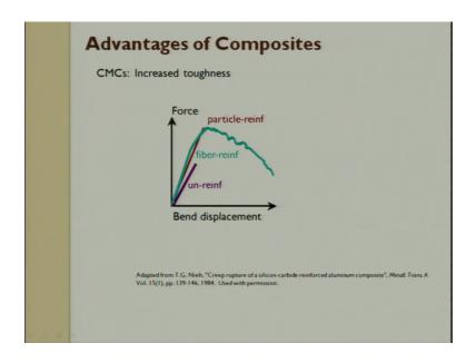
So, you can see that you have un reinforced polymer which is the bend displacement, we have we had looking into force versus bend displacement and then the next one is we are
