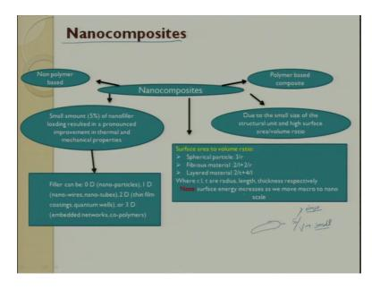
So, when you look at nano composite these are the classifications, the nano composite it can be polymer based composite due to small size of the nano particles of the structural unit and high surface area to volume ratio this we are talking about the nano. So, nano materials will have a very large surface area, but a very small volume. So, s by v so s is large and volume is small. So, here what happens is we do not talk about gravitational
