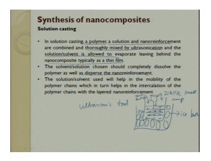
In solution casting a polymer a solution and a nano reinforcement are combined thoroughly mixed by ultrasonification. So, what is ultrasonification? We use a ultrasonic, we use ultrasonic agitator, ultrasonic tool where and which we fill the polymer. So, that tool is there. So, it tries to vibrate in 21 kilohertz with a small amplitude and creates lot
