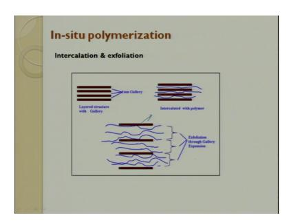
So, what I explained you is given in clear picture here. So, these are the layers. So, it is layered structure with gallery. So, now, in this layer it is all attached to each other just for schematic representation we have given the spacing, now what I do is inter calcination something flows in between and it tries to separate out a distance right. In exfoliation what happens this distance is further enhanced and we separate out layer by layer by layer.
