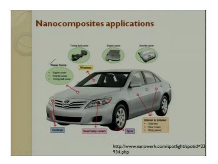
So, some more examples power train, timer belts, engine cover, inverter cover, coatings, headlamps, tires and then interiors all these things are made out of nano composites and they are finding it applications.
