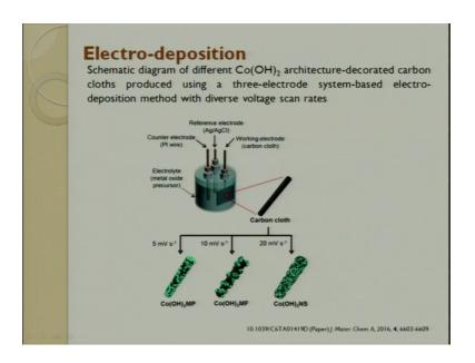
So, this is another process which is electro deposition. So, in electro deposition, deposition means I tried to deposit nano materials on top of polymer and try to make a composite out of it. So, the electro deposition the schematic diagram of a different CO OH twice architecture de corrected carbon cloth produced using a 3 electrode system based electro deposition method with diverse voltage scanning rates can be done.
