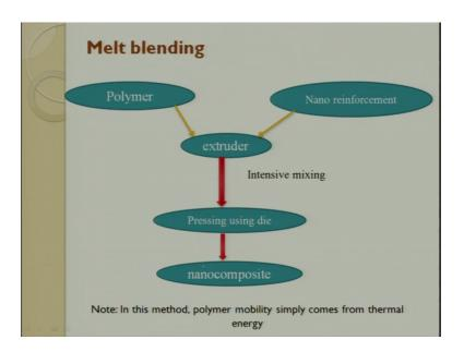
So, the melts blending is the other process we take a polymer, we take a nano material it is extruded it is intensive mixing is happened then it is pressing using a die and then you get a nano composite in this method the polymer mobility simply comes out from the thermal energy.
