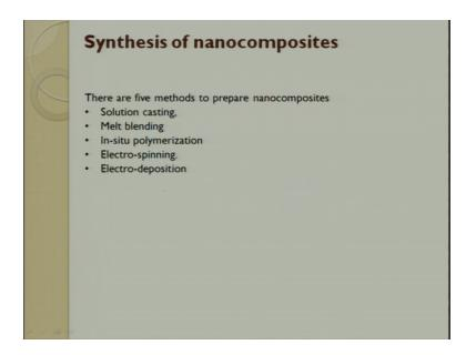
So, what are the most common synthesis route for nano composite, these are the 4 or 5 very common preparation route for nano composite solution casting, melts blending in situ polymerization, electro spinning and electro deposition, in situ polymerization when you do polymerization the particles gets generated of its own. So, these are nano in shape. So, it gets dispersed.
