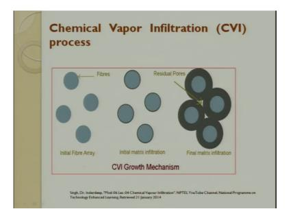
In CVI process this is how the CVI growth mechanism is there. You have initial fibre which are erase these are initial fibre erase. These are initial matrix infiltration happens right. And then what happens is this is first let us take this is one stage, and in the next
