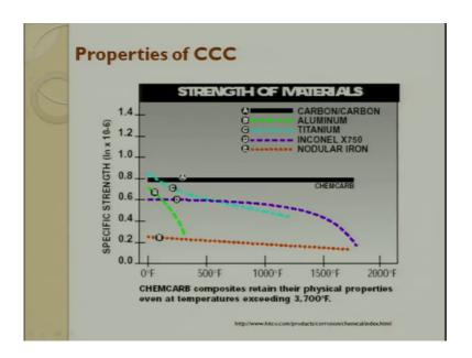
So, if you look at specific strength at varying temperatures, you can see that carbon-carbon composite the specific strength is almost constant up to 2000 degree Fahrenheit, whereas aluminium there is a decline. Titanium you can see over a period of time it is decline inconel for slightly higher temperature, and nodular iron with also there is a decline which happens over a period of time.
