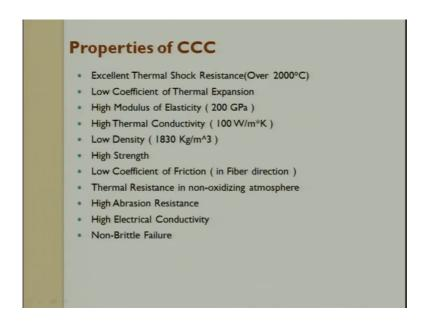
So, if you look at the properties of the CCC composite. It has excellent thermal shock, low coefficient of expansion, high modulus high conductivity, low density high strength, high coefficient of very low coefficient of friction, high resistance in non-oxidized atmosphere, high operation resistance electrical conductivity. And non brittle fracture, these are some of the properties which are good for carbon-carbon composites.
