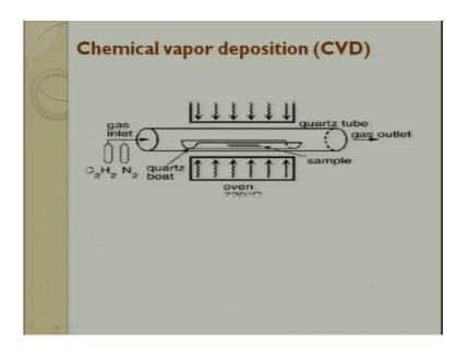
In a CVD process we use gases, and then we use a career gas. It is passed through a furnace and where and which there is a maintained temperature of 720 degree Celsius. This is a quartz tube and there is a quartz boat which is their parent with sample is given by CVD the carbon is getting deposited on the fibre and we make a carbon-carbon composite. In this process this is quite slow and second thing is here there is a possibility of other impurities coming from.
