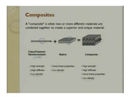
So, here a composite you are trying to use fibre, which is made out of which is made out of carbon material. Then you will also have a matrix which is made out of carbon material, these 2 put together we try to get a carbon-carbon composite. The function of the filament here is to give high strength high stiffness, and it also tries to give you low density. The matrix it has to have good shear strength property and low density. So, you see here this is also low this is also low.
