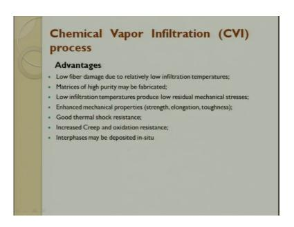
So, what is major advantage low fibre damage happens here, then highest purification can be done low infiltration temperatures are required, enhanced mechanical properties can be done. Good shock resistance happens increased creep and oxidation behaviour comes. Interface can be deposited in c 2 we want to enhance.
