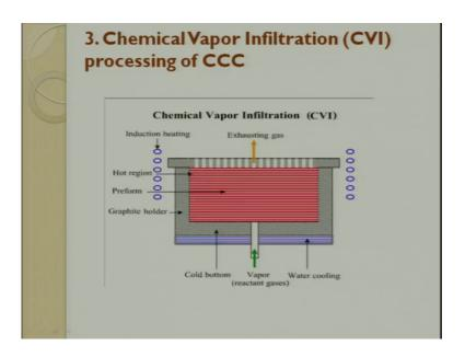
So, here through this the reactant gas is passed through. Here is the preform carbon fibre which is kept, this gas goes into reacts and then makes a carbon-carbon composite when they reacts. Whatever happens is only at a nation stage or in a green stage then after this it has to undergo 1 or 2 times of more graphitization. So, that the carbon-carbon
