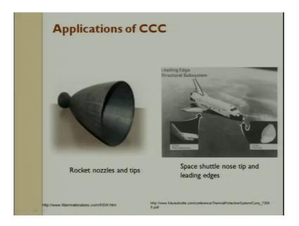
So, this withstands very high temperature. So, a space shuttle nose tip are made out of carbon-carbon composites. (Refer Time: 21:34) of very high temperature.
