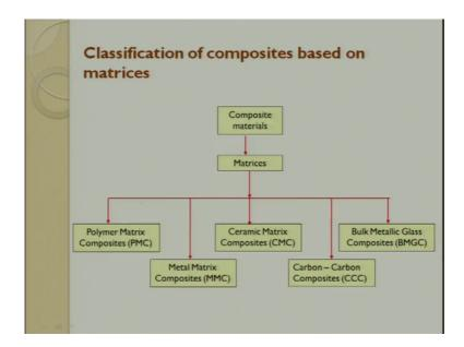
So, matrix the matrix can be polymer matrix composite, metal matrix composite, ceramic matrix composite, the most interesting and which is finding lot of applications are carbon-carbon composites. Then we also have bulk metallic glass composites. This is a next field which is coming up which is called as BMG composites. In this lecture we will more focus towards about a CC composites.
