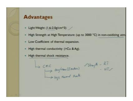
So, structures are there. So, what is the advantage of carbon-carbon composite. It is very light and weight you look at it is one point to 2 grams per centimetre cube. It has very
