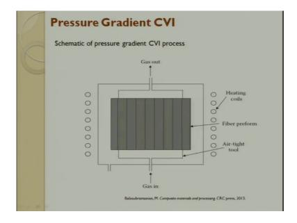
So, the schematic diagram is seen here. So, you have this is a fibre preform. This is the gas in, this is the gas out. So, you have heating coils and here it is sir tight. So, that you try to make simple geomentries out of it. So, there is a pressure gradient which is maintained such that you get the CVI done for making carbon-carbon composite.
