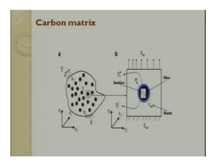
If you look at it this is a composite carbon-carbon composite, this is a carbon matrix. And these are the fibres which are used.
