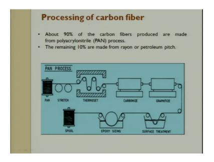
So, how is the carbon fibre prepared? So, in a pan process, we take pan and then we try to stretch the fibre pass this fibre through a thermoset, and then we try to carbonize it. Then graphitize it, then we try to do a surface treatment, then epoxy sizing we do and then finally, we wind it in a spool. So, about 90 percent of the carbon fibre which are produced today are made out of pan process. The 10 percent is made from rayon process, and this is a very well established process.
