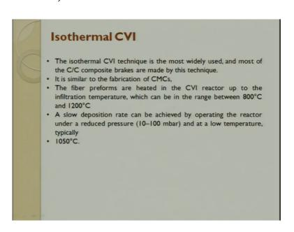
So, what is isotherm which we are discussing? There were 4 different types of CVI. So, what is isotherm CVI, isotherm CVI is the most widely used process and it is very similar to that of a ceramic matrix composite. So, hear the fibre preform are heated in a CVI reactor up to a infiltration temperature in the range of 800 degrees to 1200 degree Celsius.
