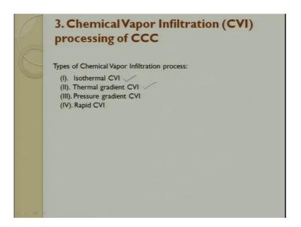
So, I said told you last time in ceramic matrix composites, we have a isothermal CVI process, we have a thermal gradient CVI process, we have a pressure gradient CVI process, we also have a rapid CVI process for making carbon-carbon composites.
