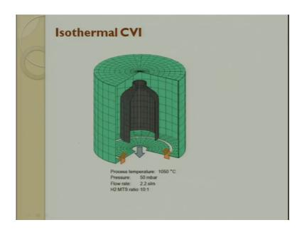
So, this is a isotherm CVI. So, you have a process temperature of 10, 50 degrees Celsius. The pressure is 50 millibar, the flow rate is 2 point 2 S L M. And then h 2 is to M t s ratio is 10 is to 1. So, here this is an isotherm we push in gas inside the furnace and we start using it.
