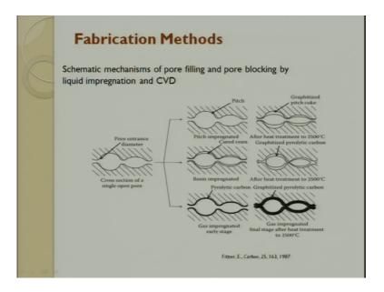
So, fabrication Method here is a schematic diagram which is given; so the schematic mechanism of pore filling and pore blocking by liquid impregnation and CVD process. So, here what we do is we these are the pores pore entry entrance diameter, and this is the cross section of a single pore.
