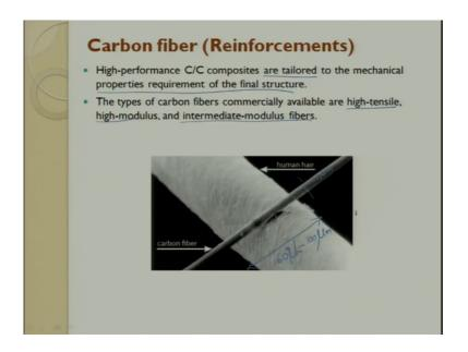
The carbon fibre which is used in the CC composite are tailored for to the mechanical properties of the final structure. So, for this the carbon fibre place a very, very important role. So, carbon fibres are having vey high strength of modulus, intermediate modulus fibre also available in this in carbon fibre. So, this is a human hair. And this is a carbon
