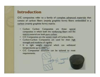
So, it is a family of complex advanced materials that consists of carbon fibre embedded in a carbon matrix. So, carbon-carbon composites are those special composites in which both the reinforcing fibre and the matrix are made out of pure carbon. They are made out of woven mesh of carbon fibre they are used for very high strength to modulus of rigidity they get.
