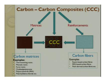
So, a matrix; so what are the different types of carbon matrix. They are thermosetting resins since can be thought of phenolic resins. You have furan resins, then oxidized
