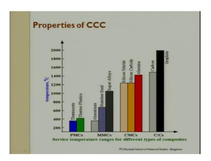
So, if you look at temperatures polymer matrix composite it can with stand a thermoset can go up to 300 or 400 degree Celsius. This can go up to 5 degree Celsius when you
