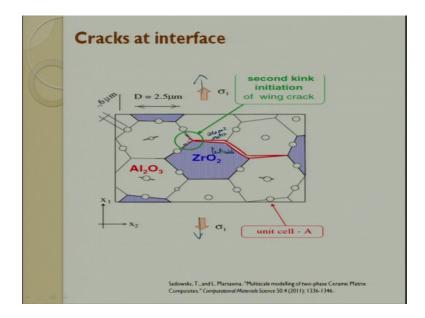
So, you can see here. So, here it again it bifurcates, and it starts growing, and this, this are the loads when they are applied, tensile load which is applied. So, you can see what happens to the crack and how does it grow. So, in all the three cases you see the important thing is, tensile is loaded, it is loaded tensile, and because of that the crack keeps growing. So, this is wing level, micro level crack, this is mesocrack, then this is secondary kink initiative for wing cracks.
