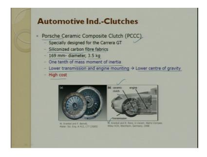
So, the Porsche ceramic composite clutches are made out of it, which is called as PCCC Porsche ceramic composite clutches, designed, designed and these siliconized carbon
