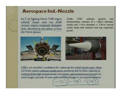
So, in the nozzle; the aerospace nozzles, which we use F 16 fighter planes right. So, the engine exhaust nozzles with five A 500 ceramic matrix composites divergent seals, which are. These are the divergent seals which are, you made out of ceramic matrix composites.
