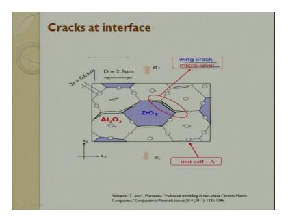
So, these are nothing, but wing cracks at micron level between the interface.
