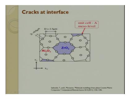
So, the cracks at interface, you can see here. This is alumina, this zirconium oxide. So, this is the diameter of the, there are saying 2.5 microns, and this is the small reinforcement which is there.
