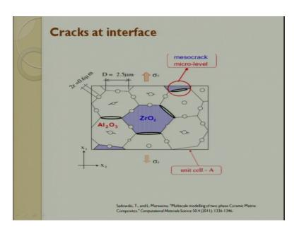
So, these are mesocrack, these are wing crack, micro level crack which happens and the crack keeps growing. So, you see beautifully that crack keeps going from here to the next crack. And the other thing is the micro level crack, between the grains it can have, and the last one is the second king initiative of the wink crack.
