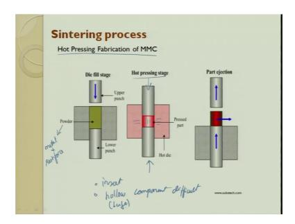
So, in hot pressing; what we do is we try to put up powder. So, in this powder what we do is we try to take a metal powder as well as the reinforcing powder we try to mix them properly and then we try to put it in a die and then compact it we try to put in die and then compact. So, then what we do is we apply hot pressure hot pressing stage means we try to apply heat here pressure is applied heat is applied heat and pressure is applied and then finally, what we get is an output.
