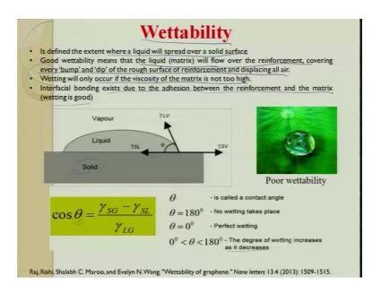
Let it be thermoset composite; let it be metal matrix ceramics which will see later. So, all these things basically depends upon a property call wettability; wettability means how good a the polymer can spread or can the matrix spread around the reinforcement. If we
