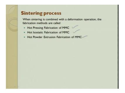
And the sintering can be done by hot pressing; it can be done by hot isostatic pressing. So, hot pressing means it is only pressing from 2 directions isostatic means with all along you apply uniform pressure. So, that you get a sound output then you can also have hot powder explosion fabrication of MMC.
