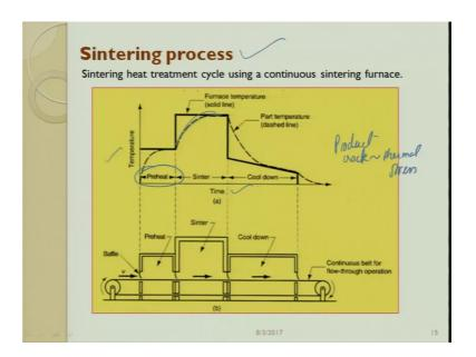
So, I told you earlier also; if you want to do a sintering process you cannot have direct ramping in of the higher temperature we divided into 3 stages. So, the first stage will be preheating. So, preheating will try to take; it was certain temperature not exactly towards the melting slightly less than a melting point we try to take the temperature and maintain it there.
