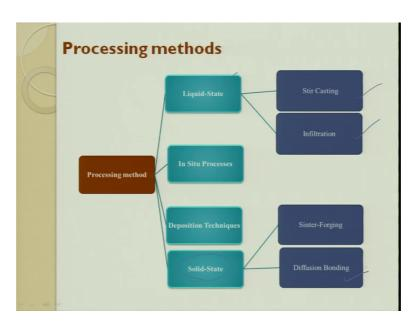
So, processing methods we had liquid state last class we covered stir casting method and infiltration method. So, now, what we will do is we will get into solid state. So, solid state; we will try to see diffusion bonding and sinter forging in solid state fabrication metal matrix composite.
