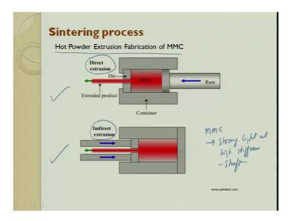
Next one is the hot powder exclusion. So, here what we do is we mix everything and then we try to do with we mixed metal particulate and then we try to apply pressure; we try to apply heat and then the pressure is given through this ram we try do an extrusion process through this. So, you can do a direct extrusion you can do indirect extrusion.
