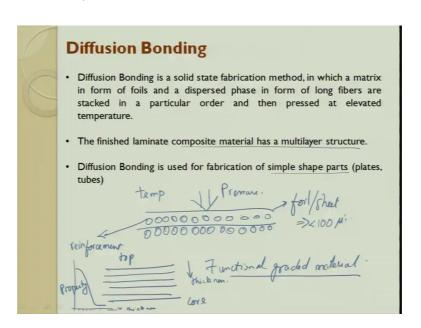
Diffusion bonding is a solid state fabrication method in which a matrix is in the form of a foil. So, we take a foil then we try to put some reinforcing agent whatever it is and then we try to have one more foil then we have reinforcement.
