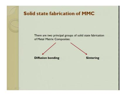
So, there are 2 principal groups of solid state one is diffusion bonding the other one is sintering; what is diffusion bonding.
