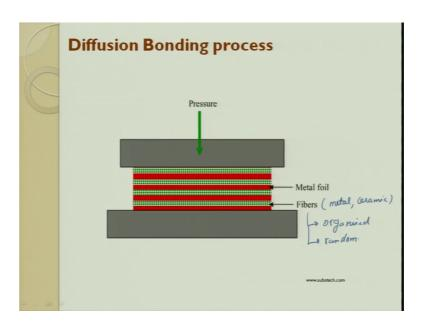
So, this can be fibers can be organized in some pattern it can be random in nature also. So, the next bounding process is called as sintering.
