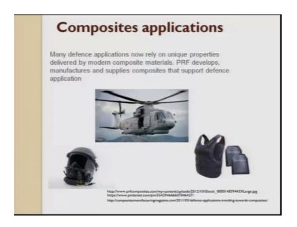
As I was talking to you about defense; helmets have become much lighter. Bullet proof jackets have become much lighter, but lighter and high performance. So, inside a bullet jacket now ceramic tiles are used. These ceramic tiles are again a composite material which has very high toughness and very light in weight, which helps the soldier without getting fatigue when he is an operation he can perform efficiently.
