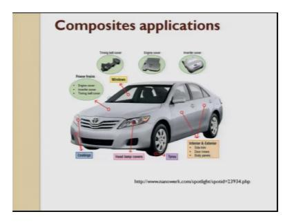
Cars, as I told earlier, today, in cars also there are lot of parts which was earlier made out of alloys are getting replaced by metal matrix composite materials, for making the car lighter stiffer and perform much higher.
