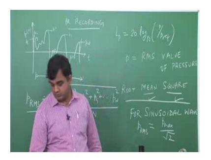
For sinusoidal waves, p RMS is equal to p max over square root of 2. So, it is important to understand that only for sinusoidal wave the RMS value of pressure is maximum pressure divided by square root of 2 this factor changes based on the shape of the wave. For this wave it may be something totally different we do not know we have to actually calculate it for the square wave it will be a different value. For a sinusoidal wave or a
