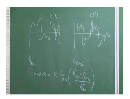
So, suppose there is 1 signal and then there is another signal. So, this is signal 1 this is signal 2 and both of these are not correlated. In this case if we have to combine the effect of these 2 signals, what we do is you add up energies, when I say energies, we can do that in equivalences by adding up the square of the RMS.
