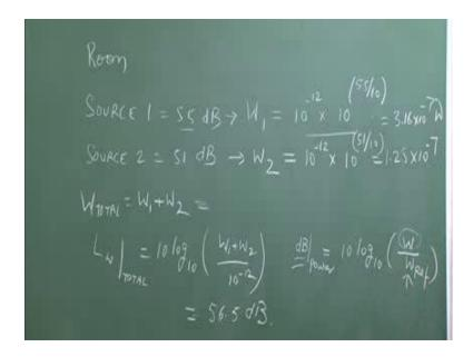
So, you have let us say you have a room; source 1: 55 dB is 51 dB. Then from here, you calculate how many; what is the power flowing out of this source. So, W1 is equal to 10 to the power of minus 12 times, 10 to the power of 55 over 10. How did I get this? I got this because I know that dB for power. This method is for power, but if you have pressure you can do it in the same way. So, dB power is equal to 10 log of 10 RMS power divided by reference power.
