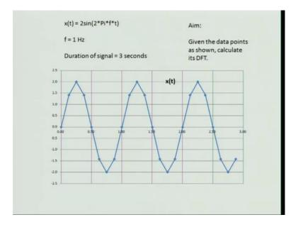
This is the value of x t. So, x t was 2 sin times 2 pi f t. The frequency of this signal I specified at 1 hertz, duration of signal was 3 seconds. X axis is time, so I have computed
