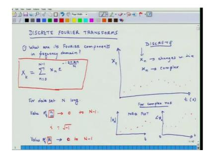
We will discuss Discrete Fourier Transforms. We will not prove whatever relations I am going to talk about, but we will directly state the results and then do a couple of examples to understand this whole concept. Suppose, I have a data acquisition system and its acquiring some data and I am going to plot this data, on the time axis we have time in seconds and on the y axis I plot values of this data and I call it x n.
