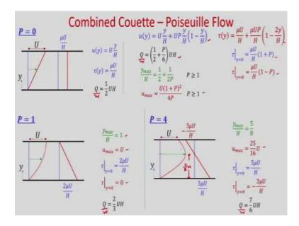
So, you can see this is our velocity profile this is the shear stress profile, and the volume flow rate is per unit width so it is Q/W is this. And bottom plate shear stress is this one upper plate shear stress is this one and for maximum velocity P greater than equal to 1 you will get
