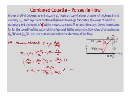
Now, let us solve two problems. First problem we will consider as 2 layer Couette flow. Already you have found the velocity profile as well as the volume flow rate per unit width. So, first problem is a layer of oil of thickness a and viscosity  $\mu_0$  floats on top of a layer of water of thickness b and viscosity  $\mu_w$ .
