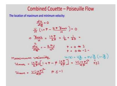
So, now you want to find the location for maximum or minimum velocity, because you can see that the flow is occurring due to shear-driven flow as well as pressure-driven flow. So, you can see that maximum velocity always it will not occur at the top plate.
