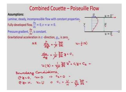
The following assumptions we will take while solving these combined Couette and Poiseuille flow. We will consider laminar steady incompressible flow with constant properties it is a fully developed flow. So,  $\frac{\partial u}{\partial x}$  is 0 and; obviously, the plates are infinite.
