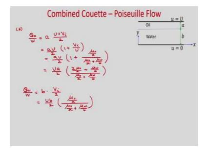
Next, we need to calculate the volumetric flow rates. So, you can see that as the velocity profile is linear, so you can write the volumetric flow rate in oil per unit width is equal to the flow area is
