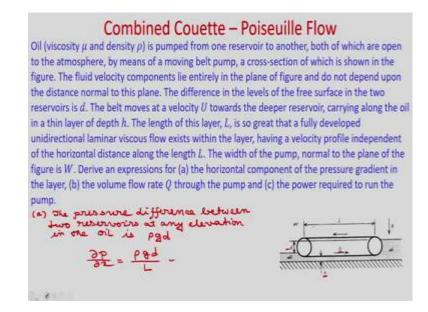
Oil viscosity  $\mu$  and density  $\rho$  is pumped from one reservoir to another both of which are open to the atmosphere by means of a moving belt pump, a cross-section of which is shown in the figure. The fluid velocity components lie entirely in the plane of figure and do not depend upon the distance normal to this plane, the difference in the levels of the free surface in the two reservoirs is d.
