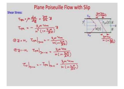
Now, let us find the shear stress distribution inside the wall and from there you will be able to calculate the wall shear stress and if you are interested you can find what is the force acting on the flat wall. So, shear stress  $\tau_{yx}$  you will just find as
