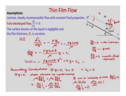
So, if you consider this is an inclined flat plate ok. So, a liquid is just flowing down due to gravity in the downward direction. So, in this direction it is going down and the film thickness is H and it is very small and we are neglecting the surface tension. So, that your surface will be straight; that means, the interface between this air and liquid, this interface will be straight and thickness will be constant as it is going down.
