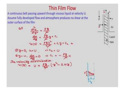
The application of this thin film flow in the vertical direction whatever special case we have discussed let us take one example. Let us consider that one belt vertically moving upwards in a viscous liquid. So, if you consider here that liquid pool is here and one belt is moving upward with a constant velocity u.
