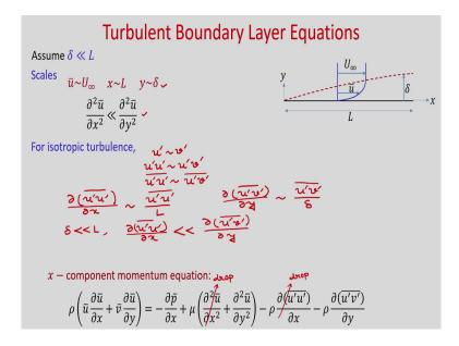
So, using this scale; obviously, you can see that del 2 u bar by del x square will be much much smaller than del 2 u bar by del y square.
