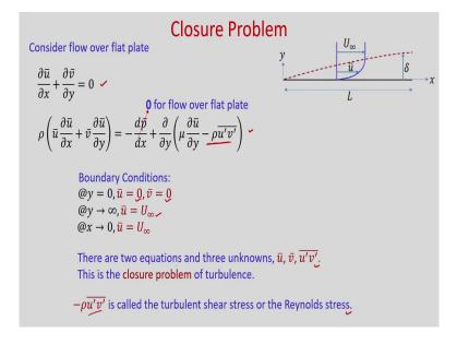
Now, we can write the simplified equations as this is the continuity equation and if we consider flow over flat plate. So, d p bar by d x will be 0. So, and we will have this term ok.
