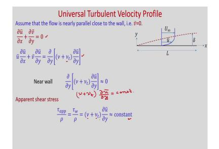
So, we can assume that v bar as 0. So, you can see that we have this continuity equation and this is the turbulent boundary layer momentum equation ok.
