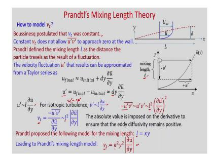
So, to model this nu t Boussinesq postulated that nu t was constant ok. So, constant nu t does not allow u prime v prime bar to approach zero at the wall. So, Prandtl defined the mixing length l as the distance the particle travels as the result of fluctuation.
