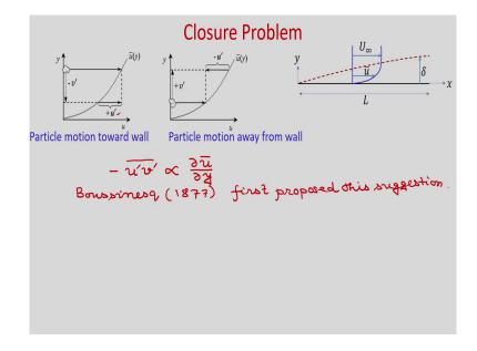
Now, question is how to model this term? So, this unknown term, let us see that whether we can model using the velocity gradient ok. Considered a fluid particle fluctuation imposed on some average velocity profile ok. So, you can see that at this location; obviously, it is having some velocity, if this fluid particle comes to this position ok in the negative y direction so;
