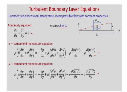
So, consider two-dimensional steady state incompressible flow with constant properties. So, this is a flat plate, flow over flat plate is taking place, this is the boundary layer thickness delta, L is the length of the flat plate, u bar is the time averaged velocity and it is varying in the boundary layer and outside we have free stream velocity U infinity. When you are considering turbulent boundary layer equations so; obviously, delta will be much much smaller than L.
