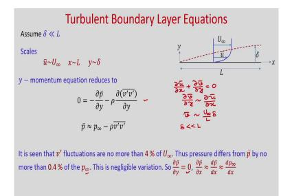
So, what is our continuity equation? Del u bar by del x plus del v bar by del y is equal to 0. So, from here you can see del v bar by del y will be order of del u bar by del x. So, v bar will be order of so, this will be u infinity ok, x is L and y is delta ok. And; obviously, delta is much much smaller than L.
