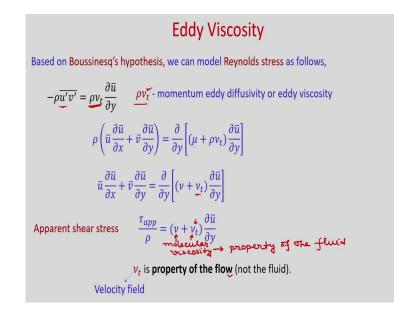
So, this was actually proposed by a Boussinesq in 1877 first proposed this suggestion. Now, based on this Boussinesq hypothesis, we can model Reynolds stress as follows. So, you can write minus rho u prime v prime bar ok. So, you can write so, this rho u prime v prime bar is proportional to del u bar by del y.
