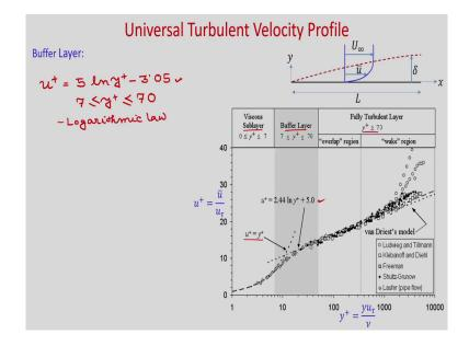
So, we can write one of these law as u plus is equal to 5 ln y plus minus 3.05and which is in the layer of 7 y plus less than equal to 70 ok.
