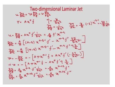
So, we have the momentum equation u del u by del x plus v del u by del y is equal to nu del 2 u by del y square and we have defined psi as A x to the power p f where f is function of eta and eta is y by B x to the power q. So, from here you can see you can write del eta by del y is equal to 1 by B x to the power q and del eta by del x we can write as y by B.
