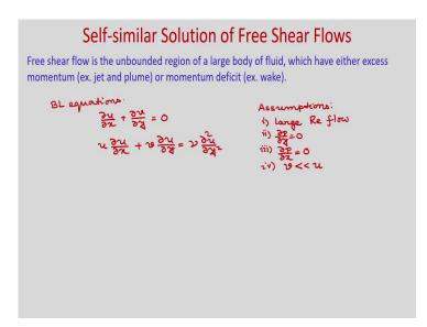
Free shear flow is the unbounded region of a large body of fluid which have either excess momentum examples are jet and plume or momentum deficit like wake. So, whatever governing equation we have derive for laminar boundary layer flows, if dominant velocity is in the x direction then those equations are valid for free shear flows. So, let us write down the governing equations.
