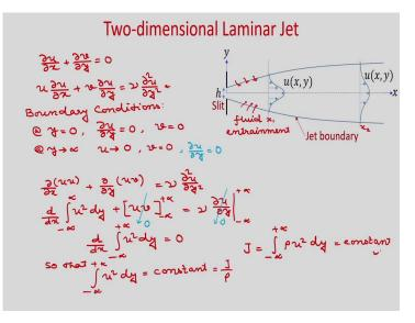
So, now we will consider two dimensional laminar jet and we will use similarity transformation technique to find the velocity distribution in the two dimensional laminar jet. So, consider this is the laminar jet and this is the small opening of height h and this is known as slit. When at high velocity this fluid will enter. So, there will be formation of jet and there will be center line.
