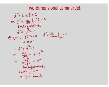
So, the equation this equation now, will become f double prime plus twice f f prime is equal to 0. Again we can write f double prime plus d of d eta f square is equal to 0 this we can rewrite like this. So, now integrating we will get f prime plus f square is equal to constant.
