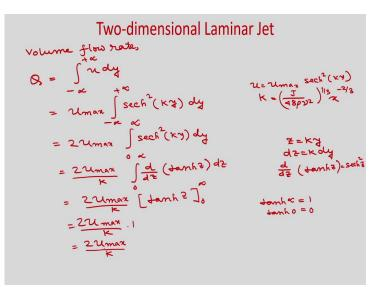
So, we can find the volume flow rate ok per unit width we are considering, because we are considering two dimensional case, so, per unit width -if you consider them Q will become integral minus infinity to plus infinity u dy and u we have written as u max integral minus infinity to plus infinity sec hyperbolic square let us write ky dy where we know that u is equal to u max sec hyperbolic square ky where k is equal to j by 48 rho nu square to the power 1 by 3 x to the power minus 2 by 3 ok.
