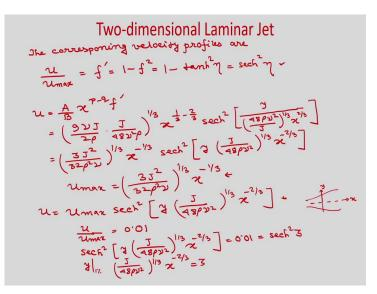
So, now we have the solution f prime is equal to tan hyperbolic eta now, we can write the corresponding velocity profiles corresponding velocity profiles are u ok by u max ok u by u max is f prime and f prime you have seen that it is 1 minus f square and 1 minus f square. So, f is already we have written in terms of eta. So, 1 minus tan hyperbolic square eta; that means, sec hyperbolic square eta.
