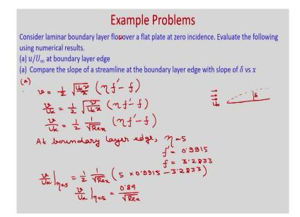
So, let us consider the next problem consider laminar boundary layer flow over a flat plate at zero incidents, evaluate the following using numerical results u by U infinity at boundary layer edge and compare the slope of a streamline at the boundary layer edge with slope of delta verses x ok.
