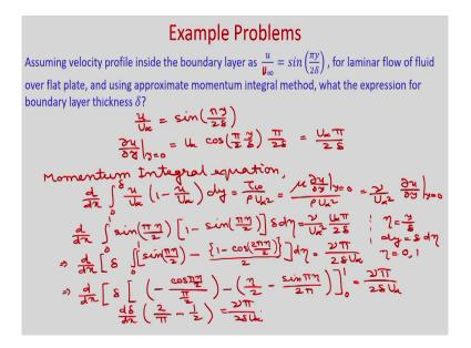
Assuming velocity profile inside the boundary layer as u by U infinity is equal to sin pi y by 2 delta or laminar flow of fluid over flat plate and using approximate momentum integral method what is the expression for boundary layer thickness delta. So we will follow the same procedure, but here velocity distribution is given u by U infinity as sin pi y by 2 delta ok.
