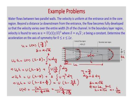
So, we can see water flows between two parallel walls, so these are two parallel walls, the velocity is uniform at the entrance. So, this is your velocity which is u and in the core region beyond a distance Le downstream from the entrance the flow becomes fully developed, so this length is Le.
