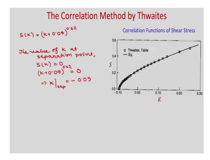
Similarly, from that table S versus K are plotted and you can see these are the square symbol this is the plot and the feet is given in this equation S K is equal to K plus 0.09 to the power 0.62. So, you can see that it is a simple, but accurate curve feet for these Thwaites table whatever it was plotted. So, this is the shear correlations given in terms of K.
