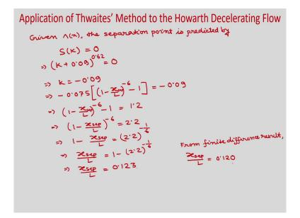
So, you can see that so for given lambda the separation point is predicted by so, S K is equal to 0; S K is equal to 0, that means, K plus 0.09 to the power 0.62 is equal to 0. That means, K should be minus 0.09 and we have the expression of K. So, that is minus 0.075 1 minus x by L to the power minus 6 minus 1 should be minus 0.09 ok.
