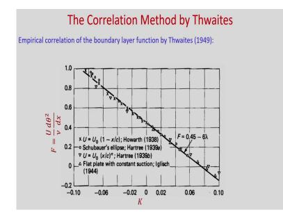
So, using different experimental results Thwaites actually tried to find this F K. You can see in this figure that for different experimental values in the in this range of K. These are the results of Howarth, then other scientist it is reported at different symbols you can see. So, this is F versus K and you can see that again this can be represented by a straight line and Thwaites proposed that F can be represented as 0.45 minus 6 lambda.
