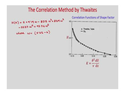
So, you can see in this plot this square symbol these are the correlation function of shape factor. So, H versus K so, this is the variation ok. So, here Thwaites proposed this simple function H K from this correlation as H K is equal to 2 plus 4.14 w minus 83.5 w square plus
