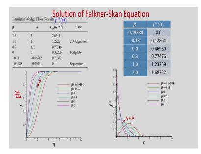
So, you can see that for the case of laminar wedge flow for different values of m; shear stress in terms of this drag coefficient and Reynolds number, it is tabulated here. So, this is the representation of f double prime 0; that means at eta is equal to 0, the del 2 u by del y square, ok.
