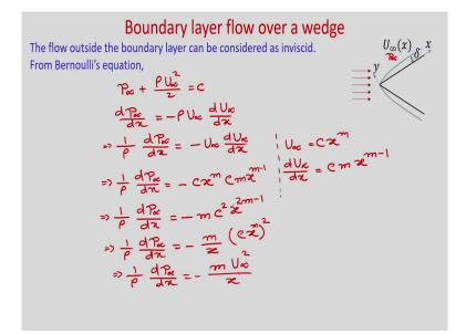
So, you know the flow outside the boundary layer can be considered as inviscid. So, from Bernoulli's equation, we can write p infinity plus rho U infinity square by 2 is equal to c. So, outside we have pressure p infinity, right. And this we have already derived in this module. So, this is the Bernoulli equation.
