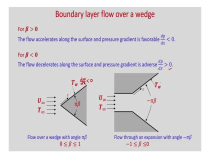
So, you can see here for beta greater than 0. So, if beta greater than 0; so this will be the situation, where situation is flow over a wedge with angle pi beta.
