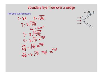
So, we will consider eta is equal to yg, where g is function of x and we have already derived that g is equal to root U infinity by nu x, ok. So, that means eta will be y root U infinity by nu x. In this case, U infinity is Cx to the power m, ok. So, if you put here, then you will get eta is equal to y root. So, U infinity we are putting Cx to the power m divided by nu x.
