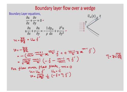
Now, let us consider the boundary layer equation with the pressure gradient term; because we are considering boundary layer flow over a wedge, so we should keep the pressure gradient
