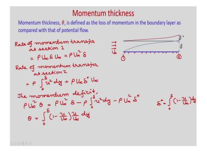
So, if we consider this as flat plate and we have free stream velocity U infinity. So, this is the stream line before the presence of this flat plate; but due to presence of flat plate, this is deflected as this. So, this is the delta star and this is the boundary layer thickness delta; so at location 1 whatever momentum you have, at location 2 there will be some deficit.
