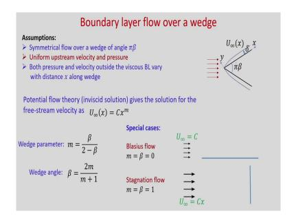
So, let us consider this wedge of angle pi beta, where you have velocity here uniform velocity. When it will pass over this wedge, so boundary layer will form from the leading edge of this wedge plate; x is the axial direction, y is the normal to this surface.
