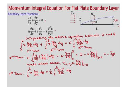
So, let us consider flow over a flat plate. So, this is the flat plate of length L, x is the axial direction, y is the normal direction and this is the velocity profile u inside the boundary layer and U infinity is the free stream velocity. So, we can write down these boundary layer equations this is the continuity equation and this is the momentum equation, where nu is the kinematic viscosity.
