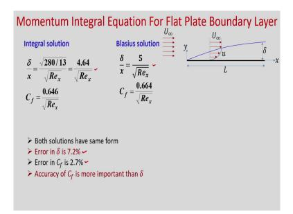
And, C f we found today from the integral solution as 0.646 divided by root Re x and in last class we found from the Blasius solution C f as 0.664 by root Re x. So, you can see that both solutions are having the same form, right. It varies as 1 by root Re x and error in delta if you see that here you are getting 5 and here you are getting 4.64.
