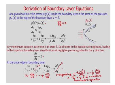
So, you can see that p is function of x only and the normal pressure gradient del p by del y can be neglected, ok. So, now we have the pressure gradient term in the x component of the boundary layer equation whatever till now we have derived, so that we can write as dp by dx, ok. So, at a given location x, if the pressure p x inside the boundary layer is the same as the pressure p infinity x at the edge of the boundary layer y is equal to delta.
