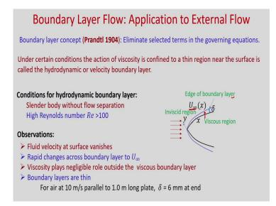
So, let us consider flow over solid surface. So, you can see, this is one surface, this is known as cylinder body and flow is taking place. Then near to the surface one thin layer
