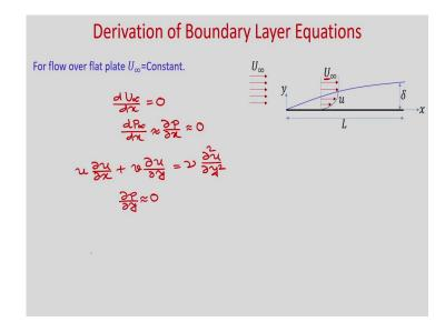
Now, let us consider a special case where we are considering flow over a flat plate. So, if it is external flow and we are considering flow over flat plate. So, the free stream velocity U infinity which is the velocity outside the boundary layer that remains constant; that means U infinity is constant.
