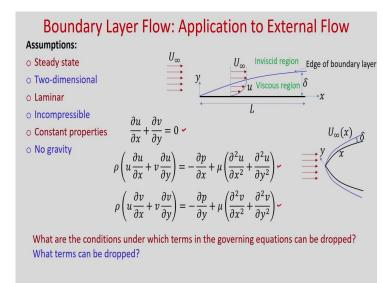
So, first let us write down the governing equations of fluid flow. So, we will assume steady state, laminar, incompressible fluid flow with constant properties; we will neglect the gravity term. So, this is the continuity equation for two dimensional case and this is the x momentum equation and this is the y momentum equation.
