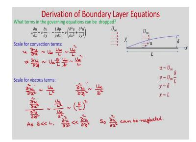
So, the next question is that, what terms in the governing equations can be dropped? So, first let us consider the x component of the momentum equations. So, these are the inertia terms, this is the pressure gradient term and this is the viscous term, where nu is the kinematic viscosity of the fluid and rho is the density of the fluid. And we have the scales as u order of U infinity, v already we have derived v is order of U infinity delta by L, y order of delta, and x order of L.
