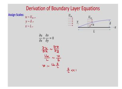
So, we have the scale for u as U infinity, y as delta, and x as L. So, this is the continuity equation. So, if you see that we can write del u by del x it will be order of del v by del y. So, now, assign the scale. So, u is U infinity, x is L order of v by delta. So, you can see that the scale for v as U infinity delta by L; but we have already postulated that delta by L is much much smaller than 1, so obviously v will be very small. So, now, we got the scale for velocity v.
