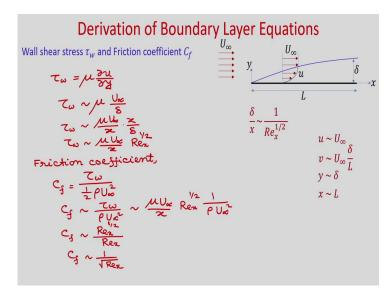
So, when we consider the fluid flow over a surface; then obviously we are interested to know what is the shear stress acting on the surface and what is the friction coefficient which is the measure of non-dimensional shear stress, so that we want to measure, ok. So, if we see that the shear stress tau w ok, we can write for this flow over flat plate as mu del u by del y, right.
