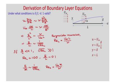
So, now we postulated that delta by L is much much smaller than 1. So, under what condition this is valid? Ok. So, for this now let us compare one inertia term with the viscous term. So, we have inertia term u del u by del x ok; each inertia term is of same order, so you can write any inertia term we can take. So, u del u by del x. So, we will compare with the viscous term. So, that will be nu del 2 u by del y square.
