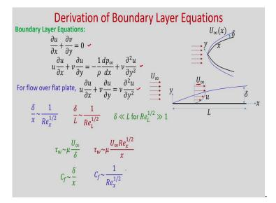
So, now let us summarize what we have studied in today's class. So, first we introduced the boundary layer. So, this is the thin layer near to the solid surface when fluid flow is taking place over a surface. German scientist Prandtl first introduced the concept of boundary layer and we used the order of magnitude analysis, which is known as scale analysis and we have dropped few terms in the Navier Stoke equations.
