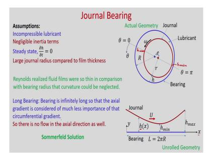
So, you can see that, this is the bearing which is known as also bushing and this is the journal, which is also known as shaft and in between we have the lubricant. So, when this journal rotates, obviously due to the shear of this journal surface, there will be flow of this lubricant.
