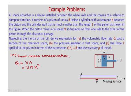
Now, let us consider the second problem. A shock absorber is a device installed between the wheel axle and the chassis of a vehicle dampen vibration. A shock absorber is a device installed between the wheel axle and the chassis of a vehicle to dampen vibration. It consists of a piston of radius R inside a cylinder with a clearance h between the piston and the cylinder wall that is much smaller than the length L of the piston as shown in the figure.
