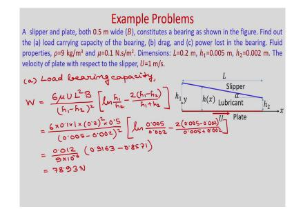
So, the first problem just I will read out first. A slipper and plate both 0.5 meter wide, constitutes a bearing as shown in the figure. Find out the a, load carrying capacity of the bearing, b drag and c power lost in the bearing. Fluid properties are given, dimensions are given and velocity of the plate with respect to the slipper is given.
