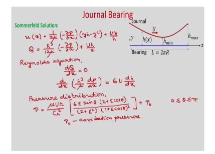
So, if you assume that this is the velocity U in the axial direction and curvature is very small; then we can find the velocity distribution u as function of y as 1 by twice mu minus del p by del x yh minus y square plus U y by h. So, from here you can find the volume flow rate Q as h cube by 12 mu minus del p by del x plus U h by 2.
