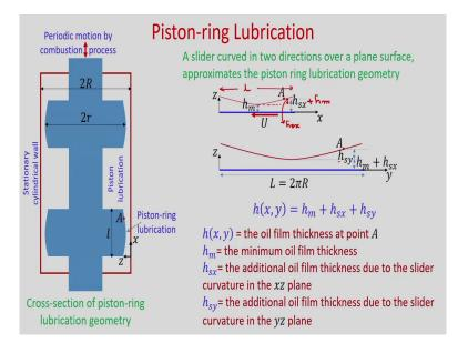
Now, let us consider piston ring lubrication. So, you know that in the combustion process, where inside the internal combustion engine; there will be piston moving around the cylinder surface and their lubrication will be there and that lubrication also we can find the analysis of this pressure using this lubrication theory.
