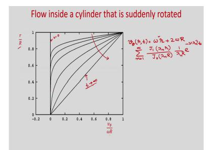
So, this problem if you solve, then finally you will get the velocity profile as v theta r, t is equal to omega r. This is the solution from the steady problem, where the cylinder is rotating with constant velocity omega plus 2 omega R summation n is equal to 1 to infinity J 1 lambda n r divided by J 0 lambda n R and you will get 1 by lambda n R e to the power minus nu lambda n square t, ok.
