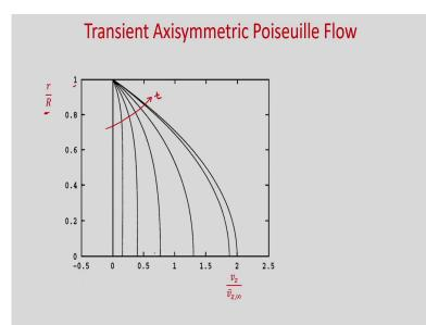
So, now, let us see the evolution of this velocity profile. So, in y axis, we have plotted r by R and obviously it will vary then 0 to 1; at r is equal to R it will become 1 and here we are plotting v z, which is your transient velocity profile and v bar z infinity, which is your steady state Hagen Poiseuille flow velocity profile, ok.
