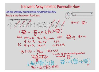
So, now you can see that this is our flow inside a circular pipe, where pipe radius is r and z is the axial direction; r is measured from the central line and we consider laminar unsteady incompressible
