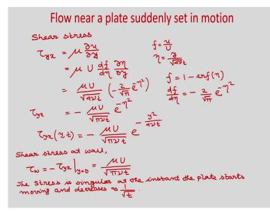
So, shear stress distribution inside the fluid domain will be just tau y x as mu del u by del y ok. So, obviously, you will get mu U, so f is u by U ok, and eta is y by root 4 nu t. So, del u by del y you can write U d f by d eta into del eta by del y. And del eta by del y from here you can write mu u by root 4 nu t.
