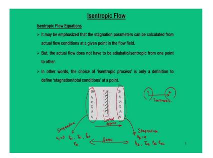
Now, when I said that in a isentropic flow field, we say that a system undergoes a change of state from 1 to 2 and when the process is isentropic. So, the essentially basic feature is that when such a change takes place 1 and 2 we can represent that change to happen in a small volume we call this as a control volume as shown is this figure.
