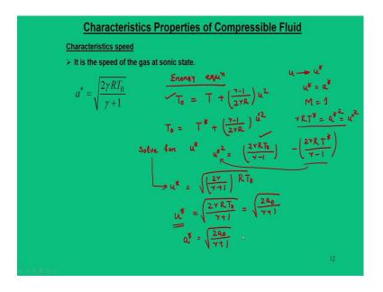
Again also we can find out same these expressions using the energy equation. So, we can know that how that energy equation is very vital in all this analysis. So, everywhere you are using this energy equations here; we will use this energy equation for stagnation temperature  $T_0 = T + \left(\frac{\gamma - 1}{2\gamma R}\right)u^2$ .
