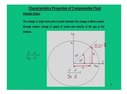
So, now let me see that when you take this adiabatic ellipse equation, how you represent it graphically. So, this is the equation of the ellipse. So we are plotting this graphically where x axis represent u, y axis represent a. We have a gas can attain maximum velocity that is  $u_{max}$  which is given by the abscissa of this ellipse or that is half of the major axis.
