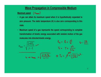
Now, when given flow field is defined as its velocity u, what is the maximum speed it can attain? So, this is we call as a maximum speed that is  $u_{max}$ . So, a gas can attain a maximum state when it is hypothetically expanded to zero pressure. So, when it is at a zero pressure, but the static temperature is also 0 that is represented in terms of Kelvin corresponding to the state.
