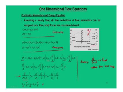
So, with these assumptions we will now move to the one dimensional flow equations. So, here we say that Q is the heat added into the systems. So, obviously we will be talking about three important equations that is what we discussed in the last module; continuity equations, momentum equations and energy equations. And all these equations are addressed through the control volume approach.
