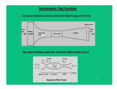
So, likewise I will just give some introduction that what are the facilities available so far. We have a low speed continuous subsonic wind tunnel, where speed range is about 50 m/s. Typical way of operation is that this is a very fundamental wind tunnel where we have electric drive that is in terms of fan and motor.
