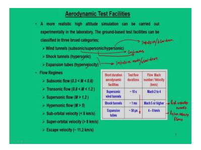
So, with this the different flight regimes between subsonic to may be hypersonic flow and then towards this hypervelocity flows. We have classified the ground based aerodynamic facilities in 3 broad categories, one is wind tunnels. This wind tunnels can be subsonic mode, supersonic mode or hypersonic mode.
