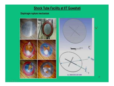
Now, another important aspect of this shock tube that when we are talking about a shock tube whether really a shock wave is generated or not. So, this is ensured through a visual inspection and we put this diaphragm into picture. So, we have a very well designed diaphragm that is a circular diaphragm, and it has a kind of a groove which is triangular grooves, something of this sorts along this depth.
