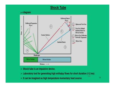
So, likewise I have explained here that shock tube it is a laboratory tool for generating high enthalpy flows for deviation of 1 to 2 milliseconds. So, it can be imagined to be high temperature momentary heat source. Here also another version of the diagram that explains about different regimes 1, 2, 3, 4 and it is the  $\Delta T$  which is this.
