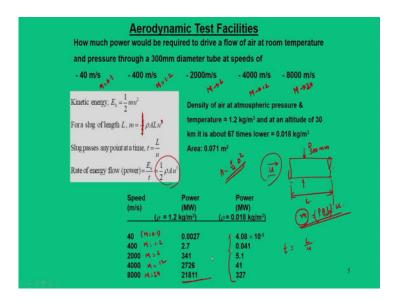
But before you move for the aerodynamic facilities, in fact, design of any facilities requires a lot of power. So, when you talk about aerodynamic ground base facilities, we must know that what type of power requirement we need to establish such facilities. A simple calculation will tell us that what type of parameters or power that we require.
