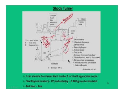
Now, I will move further to give some introduction to a shock tunnel. So, we discussed about the shock tube exhaustively. Now, a shock tunnel is nothing but we attach a nozzle and test section. So, we have two parts here, one is tube part like we have a shock tube part and we have tunnel part.
