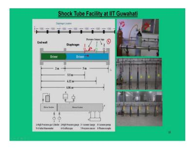
So, likewise we have a shock tube facilities at IIT Guwahati. And this is a 7 meter shock tube driver and driven, we have mounted 3 pressure sensors. You can see that the driver gas is filled with high pressure gas. In this photograph here, this particular cylinder refers to helium; this particular refers to nitrogen; that means the driver gas can be helium or nitrogen.
