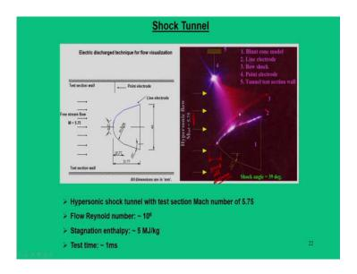
So, what we see here is that a model which is mounted in the test section. So, this entire domain is the test section wall, on the test section wall there is a point electrode, and matching to this a line electrode is embedded on the model surface.
