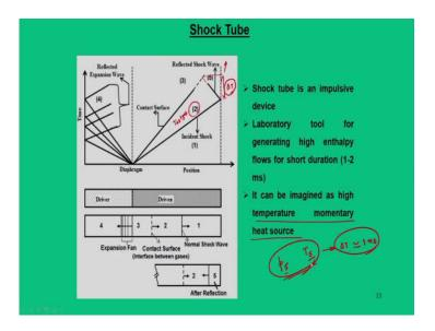
But how to quantify it? Means, which is shock wave, which is expansion wave? So, to do that a simple diagram what we call as x-t diagram is plotted; it is a kind of a distance timing diagram for a given shock tube.
