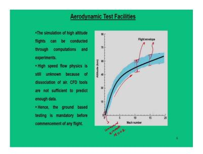
So, based on this we can have a altitude Mach number plot that way if you want to go at higher Mach number we have to increase the altitude. Now, here the aerodynamic challenge comes into picture because at low subsonic speed, even in fact the commercial aircraft this is the location for which we have commercial aircraft flies.
