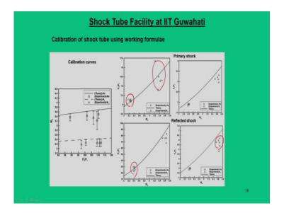
There are variety ways that we can plot the calibration curves of Mach number versus rupture pressure ratio, we can have primary shock,  $\frac{p_2}{p_1}$ ,  $\frac{T_2}{T_1}$ , we have reflected shock  $\frac{p_5}{p_1}$  and  $\frac{T_5}{T_1}$ . And if you see that the solid lines indicates the theoretical curve and the the points that we are looking at, these are the experimentally measured points. So, in some cases our predictions are under predicted, it all depends on the accuracy in the
