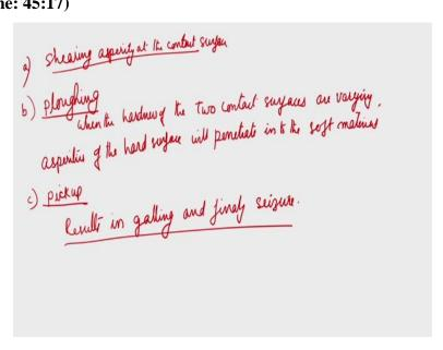
So, coming to that when you look at, how these lubricants help or how this friction is going to play an important role. Let us look at that so there are contact between the work piece and the surface. So, when the film the lubricant is added ok. See, if you just assume that there is going to be a relative motion between the work piece and the surface. So, when it comes in contact with each other the asperities you know they will come in contact first.
