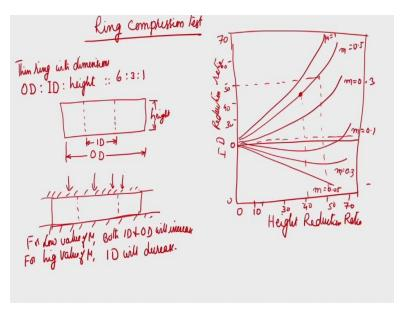
So, this ring compression test has been widely accepted. Here you take same size of a ring but with a ring with thin ring. You take large number of samples with the dimensions outside diameter is to inside diameter is to the thickness of the ring means, not thickness, the height of the ring. so if it is in the ratio 6 is to 3 is to 1. Because, this is a universally accepted practice, it is a standard which is being used.
