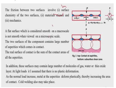
So, when you talk about the sticking friction between two surfaces, you will find that it involves one is the surface chemistry of the two surfaces. Second is the material science and so combination of these mechanics also all those are coming into picture. So, if you look at say two phases are matching, though it may be very highly polished surface like a mirror polish you are getting. And then, you may find that okay the surface is very smooth.
