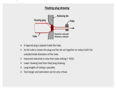
Now to overcome that part a very schematically drawn. There is a floating plug drawing. So drawing tube drawing using floating plug. So in this case also in every case you need to have this is a sectional view. In every case you need to have hollow tube as a starting material okay. But then the tube diameter is getting reduced. So here this floating plug is kept here. Normally this will be in a vertical condition.
