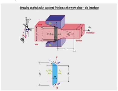
Now let us come to the analysis so your mechanics of this metal working. So maybe this is similar to that what we discussed in the mechanics of metal working. But there now we just discussed for the case of a slab method where homogenous the rod necessary for just to homogenous
