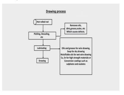
Now if we look at the drawing process the material which you are getting is normally obtained in the hot rolled form. So that hot rolled form means that in general residual stresses and other things are minimized and the material is soft. If it is cold rolled you know the material will get to work hardened and then your drawing stress will be very large not only that there will be a maximum limit for the reduction which can takes place.
