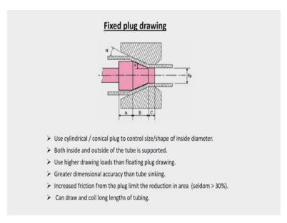
The second type of tube drawing is drawing using a fixed plug okay. So here the internal surface and the external surface both are supported. So external support is external surface of the pipe is external part of the tube is supported by the die. So here it is supported by the die and the internal part there is a fixed plug which is stationary okay. In this case these two things are there, so you will find that these 2 surfaces are supported.
