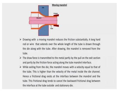
The last case is a moving mandrel okay. So drawing with the moving mandrel reduces the friction substantially this is another. A long a mandrel is there which is generally a long hard rod for a smaller diameter it may be wire also that extends over the whole length of the tube. It is drawn through the die along with the tube. So you will see that in the mandrel and the piece is held together initially you insert it and with the gripper you are fixing it and you are pulling this to together.
