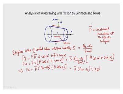
So here this is the deformation zone because it is a tapered cylindrical piece. So this is assumed to be the deformation zone inside the where the metal is radial deformation. So your initial cross sectional area Ab is there and final cross sectional area is Aa is there okay and you are pulling this
