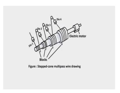
Now because many times see either you can have it in a serious arrangement which is kept there from one end to the other when it passes through that as we have shown here see in this case. So here now what happens is that, it will just a series of dies are kept and it will be pulled. Otherwise you can have it on a stepped-cone multipass wire drawing.
