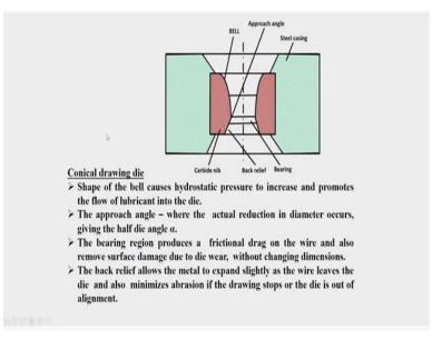
So when you look at that the die for drawing generally it is a conical drawing die which is used and this many times when the size of the wire is very small you know it becomes very small in diameter. This is a exaggerated view of a die assembly okay. So you will find that because there is a very high worker hardening which is taking place when deformation is taking place in the deformation zone.
