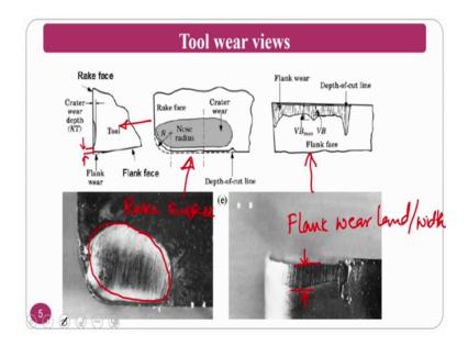
So, this is the crater wear depth normally this is the crater wear which takes place on the rake surface this is a flank wear.
