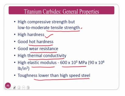
The high compressive strength normally general properties if you see high compressive strength, but low to moderate tensile strength this is problem, but you have a compressive strength is very high. So, normally it will be very good. So, high hardness and good hot hardness I said at a elevated temperatures.
