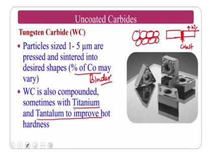
First we will see the tungsten carbide. The particle sized 1 to 5 microns are pressed sintered into the desired shape and percentage of cobalt may vary. Cobalt is a binder basically ok.
