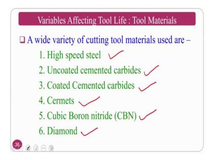
So, the wide variety of cutting tool materials used are one is a high speed steel, uncoated carbides, coated carbide, cemented carbides, cerements, cubic boron that is nitrate that is called CBN tools and the diamond tools these are the some of the materials. Apart from this many materials are coming up at the same time many materials are invented for coating on this material ok. So, these are all we will some of the things. We will see the history of the cutting tool materials.
