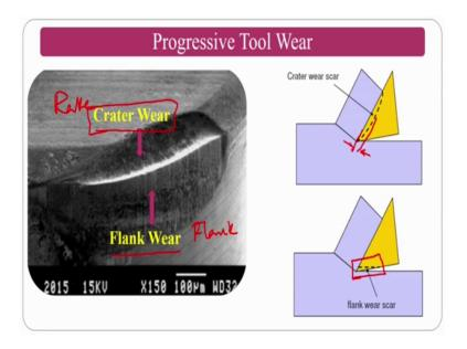
Just it if you see to the introduction to the progressive tool wear. There is a another tool wear that is called catastrophic tool wear which I am not a discussing it catastrophic tool wear is normally sudden breakage.
