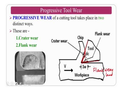
This is a progressive wear, now you can see how it takes place on the machining process we have seen previously. So, now, you see this is the cutting tool basically, in this cutting tool because of the chip motion you can see this is the crater depth that takes place because of the workpiece interaction normally abrasion there comes the flank wear. This is called the flank wear.
