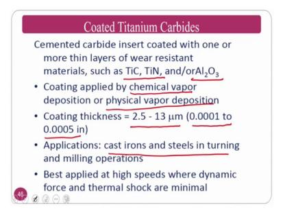
So, why the coating is required? Cemented carbide insert recorded with one or more layers normally tungsten carbide tools are not good for the steel based workpieces and all
