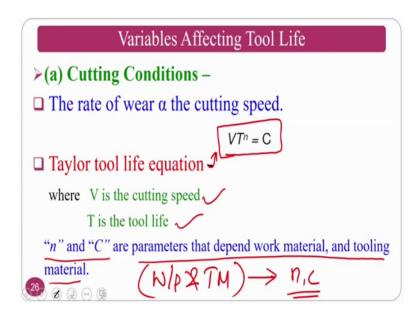
So, the cutting condition the rate wear and the cut is proportional to the cutting speed that is V T power n equal to constant this is called Taylor tool life equation. So, whenever you see this Taylor tool life equation V T power n equal to constant where the V is cutting speed, T is the tool life and n and C are the constants ok.
