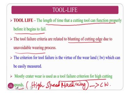
So, the tool life, tool life normally can be defined in many ways. You can see the length of the time that cutting tool can functional proper before it begins to fail ok. So, it is performing its own function, it is a machining operation. So, if it is fake; that means, that my I have to change my tool; that means, that this is my about my tool life one wear.
