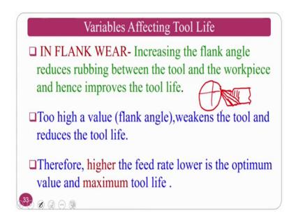
In the flank wear increasing the flank angle reduces the rubbing action between the tool and the workpiece hence it improves the tool life. This is the workpiece, this is the flanking angle ok, this is the flank angle which helps from the rubbing action. If I give the 0 flank angle what will happen? If I give 0 flank angle it will completely rub again is this one.
