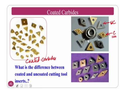
We see the coated carbides, normally coated carbide what is the difference between coated carbide and uncoated carbide. Normally these are the coated ones ok. How what is the difference normally if you see? This is the difference, this is the uncoated one this is the coated one ok. So, you can see normally it is the gold color normally the coating is done on this one ok.
