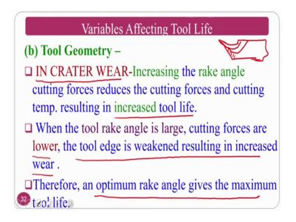
So, the tool geometry if you see normally the in crater wear. So, in the crater wear increasing the rake angle cutting force reduces and cutting forces and the cutting temperature resulting in increased tool life. Now, what I mean to say if I increase the rake angle my tool chip will be smoothly flows at the same time forces will reduce if the
