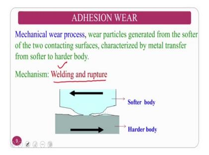
So, the next one is adhesion wear the, mechanical wear process wear particle generate from the softer and to contacting surface characterized metal surface and mechanism is welding and rupture ok. So, basically whatever here welding and rupture is the tool wear mechanism ok.
