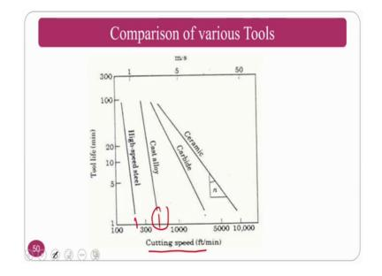
So, the comparison of various tools if you see the cutting speeds if the cutting speeds versus tool life high speed steel will have very low range of cutting speeds then the cast alloys which I have not taught then the carbides and the ceramic that is cermets and all those things. Diamond will follow next; CBN followed by diamond will come ok.
