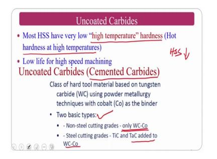
So, we are going for the uncoated carbides. The second variety is most of the HSS the basic problem is high temperature hardness is very less; that means, that hot hardness at elevated temperatures or the hot hardness is low. So, if at all I want a machine a hard
