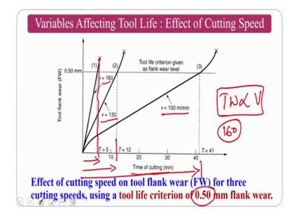
So, if you see the time of cutting versus tool flank here the effect of normally I see at know this V T power n equal to constant if you see 3 cutting velocities if ok. So, one velocity is 100 meters per mm, and 130 and 160. If you are going to increase the speed the cutting time and the for a less cutting time the tool flank wear will increase. So, this shows that tool wear is proportional to your cutting velocity ok.
