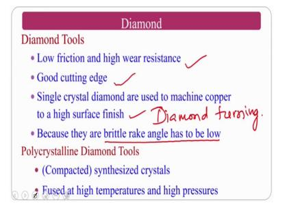
So, diamond normally will be the polycrystalline diamond and single crystalline diamond will be there normally these diamond do not think that these are the diamond that people wear or something. This is the artificial diamonds. Low friction high wear resistance good cutting edge and the single crystal diamonds are used for machine copper to get high.
