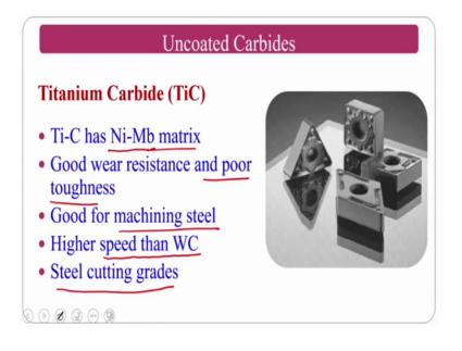
Next we will go for titanium carbide ok. So, in the titanium carbide tic nickel molybdenum matrix will be used. This is steel grades, normally previous one tungsten carbide which we are using is a non steel grades where if at all we want to use the nonferrous based those can be used.
