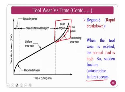
The third region that is called a rapid breakdown, when the tool wear exceeds its normal load high, so sudden fracture that is called catastrophic failure occurs this is nothing, but the failure region ok.
