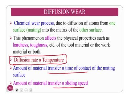
So, you can see whenever the chip is flowing on this and at high temperature normally the machining temperature gradual diffusion of atoms which are lying on a beneath of the chip gradually goes and sits on the tool surface; that means, that we will go into the tool surface that is nothing, but the diffusion.
