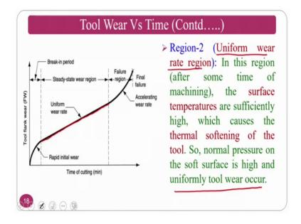
In this region after sometime the surface temperatures are sufficiently high which causes the thermal softening of the tool so the normal pressure of the surface soft surface is high and uniformly wear takes place. That means, whenever you have the sharp cutting edge is gone now your sharpness radius is increase.
