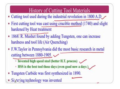
If it is the cutting tool was used during the industrial revolution that is 1800 AD. The first tool was cast using crucible method and the slight hardened by the heat treatment method normally. So, it is developed by the crucible method.
