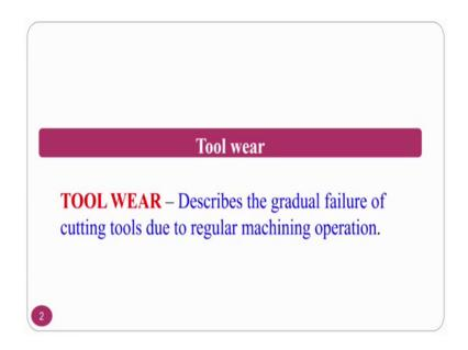
So, the tool wear, normally if you see the tool wear it describes the gradual failure of the cutting tool due to regular machining because it is a progressive wear basically. So, it describes gradually how atom by atom or molecule by molecule are the amount gradually it will goes off that is what the progressive tool wear is.
