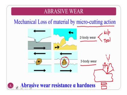
Anyhow I will come in detail about all these things that the mechanical loss of material by micro cutting action normally if you see this is to explain you what is abrasion wear. We have just taken the example of the micro cutting action.
