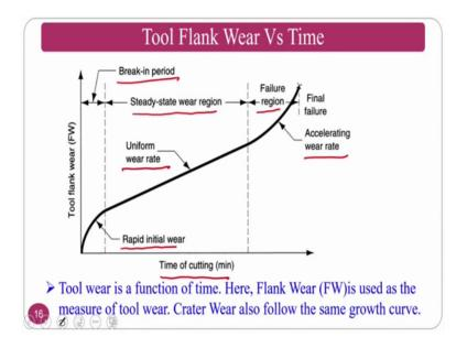
So, if you see this one the time of cutting versus the tool flank wear normally to similar trend the crater wear also follow. So, I am just touching about the only the flank wear. I will also explain you why I am touching only the flank wear because the flank wear is the criteria that people can easily measure, but the main reason is the tool life criteria basically takes from the flank wear only.
