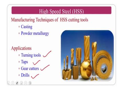
So, another one is normally these are manufactured by casting and powder metallurgy technique. So, the applications it can be turning tool, taps, gear cutting, drills and all those things ok.
