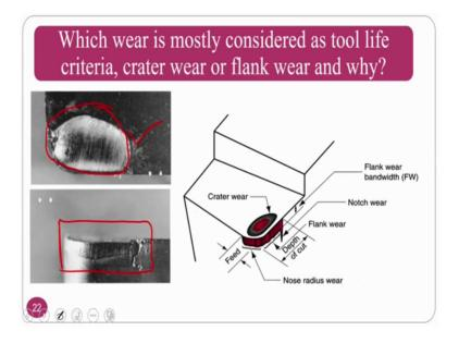
So, why the flank wear? Whenever the machining operation is taking place crater wear takes place on the rake surface and the flank wear takes place on the flank surface and the flank surface is the surface which will be in contact with my final product. So, whenever customer ask me I have to give you a product to him in a good size, good tolerance good surface finish and all those things. If my flank wear is disturbed or the
