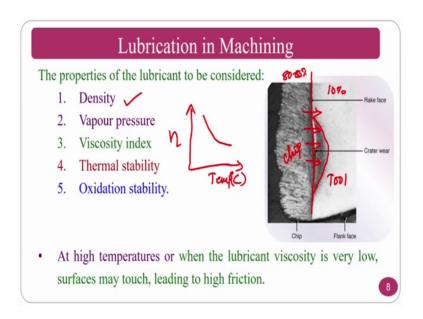
The properties of the lubricant as I was telling you if as a manufacturing engineer my aim is to send that a cutting fluid or lubricant between these two surfaces; If I can send between these two surfaces that is good for my machining so that the tool wear do not come this is the crater wear that is coming on this one it is called this is a tool since this is chip basically ok.
