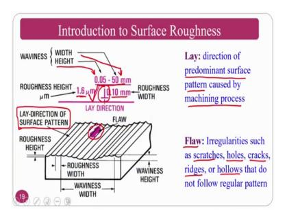
Now, we will come to what is a lay. So, lay in the previous one which is called it is a predominant direction of the surface roughness ok. So, or predominant surface patterns caused by the machining process is nothing but the lay ok. Flaw, normally flaws are nothing, but if you see here a flaw is there this is the flaw is nothing, but the scratches holes cracks ridges or a hollows that are presenting on the surface which are not as a part of machining process ok.
