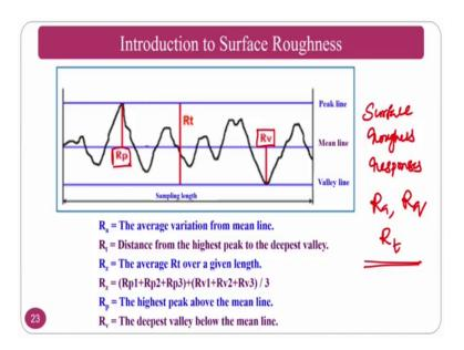
The other parameters normally if you see R p that is mean line to the maximum peak and R v mean line to the minimum value, that those are the two things R p is nothing, but the maximum peak to minimum value that is R p plus R v, this is maximum peak to minimum value.
