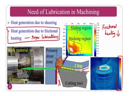
So, need of lubrication if you see the need of lubrication heat generation by the shearing that is what I am talking about a shearing, plastic deformation, severe plastic deformation, this is a major culprit generates the heat that by conversion of mechanical energy into the thermal energy. The second one is heat generation due to frictional heating that is what I was talking about which you can eradicate by the action of lubrication ok.
