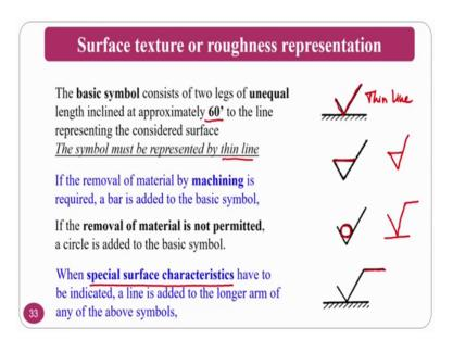
So, the surface texture or the roughness representation, so the basic symbols of the surface roughness representation is like this. If you see the basic symbol consists of two
