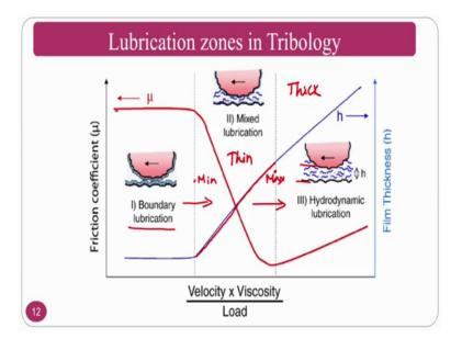
You can also see a friction coefficient how it will drastically goes down and the film thickness increases both are con converse to each other. If you see the coefficient of friction in the value lubrication because of the mating surfaces two mating surfaces are there because of the two mating surfaces of chip as well as tool the it will be very high coefficient of friction is very high.
