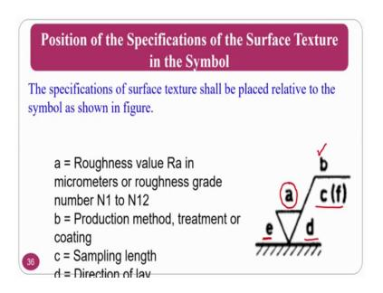
That is overall if at all I want to mention how I will mentioned the surface roughness value R a is this one the what I have the roughness I want to mention. The production method or a treatment or a coating assume that I want to go by the lay that is turning process I will mention in place of b, and c sampling length and d is direction of the lay ok. What are the allowance that I want to give I can give here ok.
