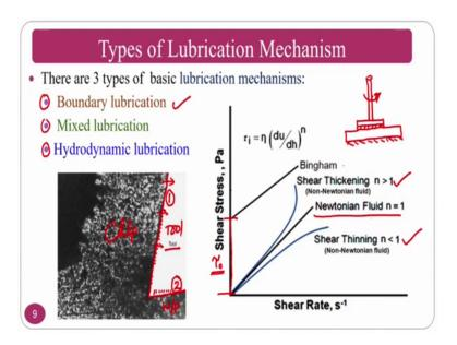
So, types of lubrication if you see one is a boundary lubrication, second is a mixed lubrication and third one is hydrodynamic lubrication these are the 3 lubrications are there ok. Why I am talking about these lubrications? I need in the two zones flank surface and workpiece, this is called workpiece region. This is chip, this is any how tool is there I need to lubricate these regions ok. This is the one region, this is the second region ok.
