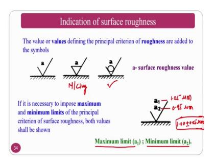
So, if the values defining the principle roughness is an added normally if you are having a surface roughness value normally if you represent the surface roughness value is a you will represent like this if you are representating the surface roughness by machining process you represent this one. And you should not remove any material, but I want the surface roughness value a then this is the process this is what you want to explain, ok.
