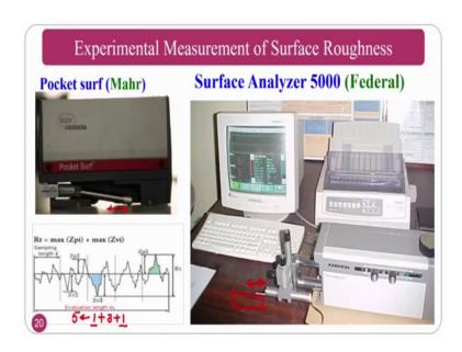
Experimental measurement normally how do you measure? So, there are two things if you see few years back like ten to 15 years back we used to have the contact sur type of surface profile emitters. For example, pocket surf is the one of the thing that is developed by mark is one of the companies.
