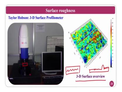
You can see the Taylor and Hobson where this is a eyepiece, you can keep your workpiece here and you can just put the it works on the interferometry principle there is a white light interferometry method it will use just it will passed and it will receive this and it will give you the 3D view of the surface roughness.
