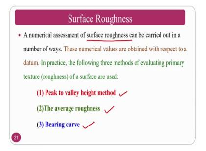
So, the surface roughness it is a numerical assessment of surface roughness can be carried out by the number of ways one is the numerical values are obtained with respect to a data ok. So, there will be a data normally according to that normally you will take. So, the following 3 methods are there, one is a peak to valley method and average roughness method and bearing area curve method ok.
