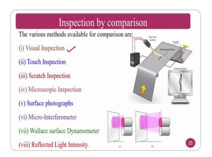
So, inspection by comparison normally visual inspection, touch inspection, scratch inspection, microscopic inspection, surface photographs, micro interferometer, Wallace surface dynamometer, reflected light intensity.
