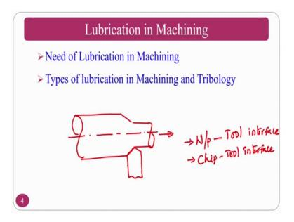
So, we will look into two aspects whenever we talk about the need of lubrication and types of lubrication. See I am talking about lubrication ok. So, I am not talking about the cooling aspect. So, why I am talking about the lubrication is whenever there is a friction between the workpiece and tool.
