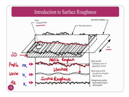
So, introduction to the surface roughness, the surface roughness if at all if you have a 3 disc space if you just see there are three things one is profile roughness, waviness, and roughness surface roughness ok.
