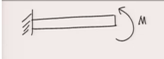
Figure 7: A bending moment M applied at point 2 instead of force P being applied at point 1
