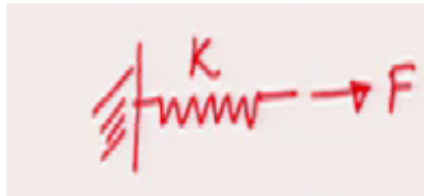
Figure 5: A spring clamped at one end is stretched by a force F .
